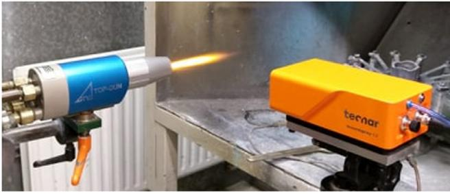
Fig. 3. Accuraspray 4.0 system in operation with an SHVOF thermal spray gun.
