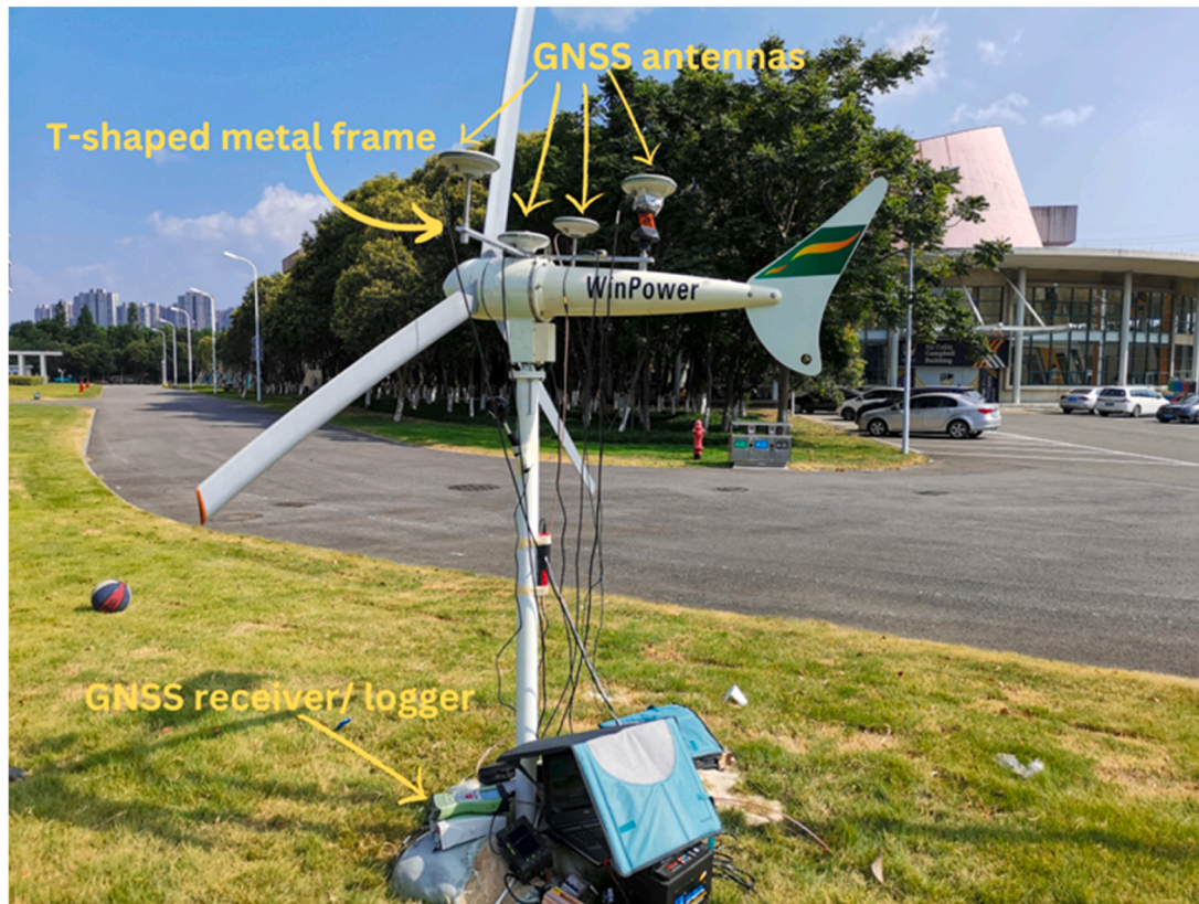
Fig. 1. The wind turbine and the layout of the GNSS antennas as mounted for the first experimental session.
