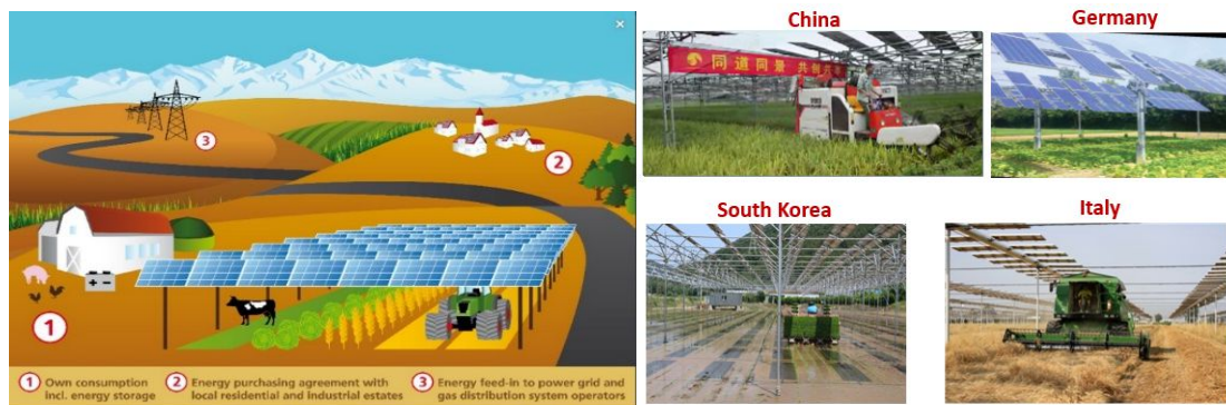
Figure 1a: basic principle of APV, Fraunhofer Institute ISE; 1b: current solution for agriculture photovoltaics by implementing mosaic type of structures carrying solar panels high above the farmland
