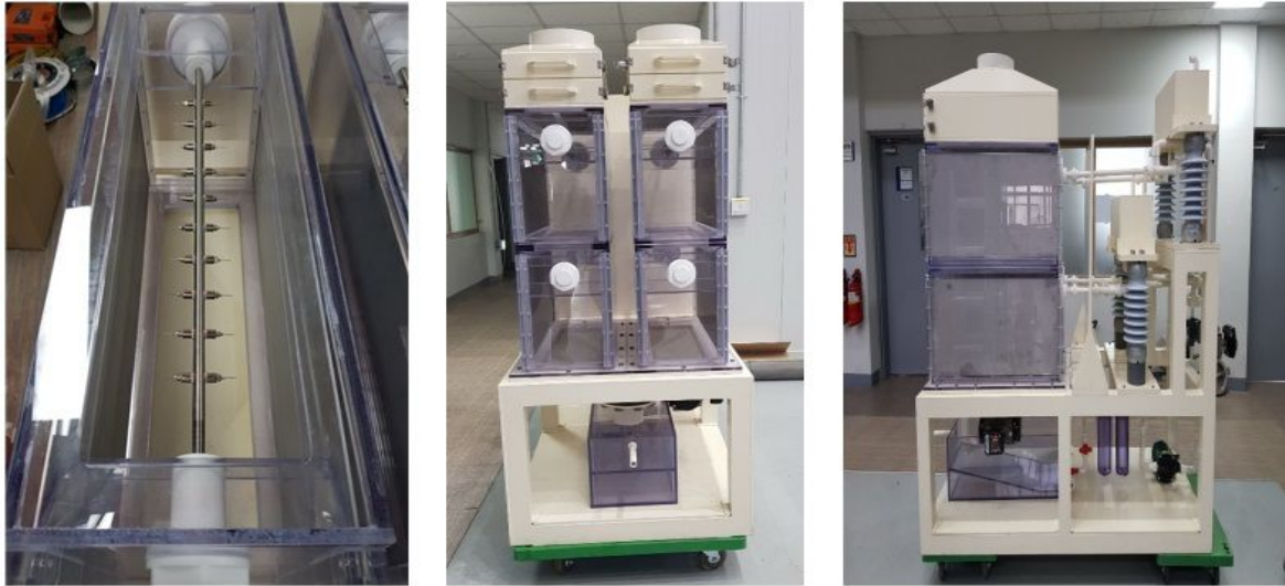
Figure 2: Prototype of the modular electro-spray precipitator
