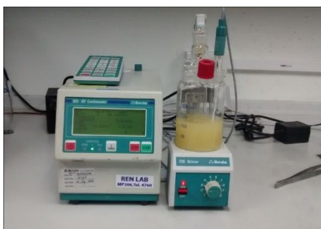
Figure 12: Metrohm, KF 831 Karl Fischer Coulometer, Renewable energy lab, MTEC
