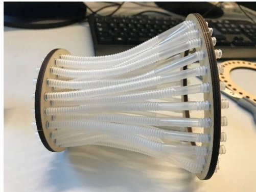
Figure 3: The straw heat exchanger core
