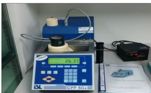
Figure 5: ISL, CPP 5Gs automatic cloud point, pour point analyser, Renewable Energy Lab, MTEC
