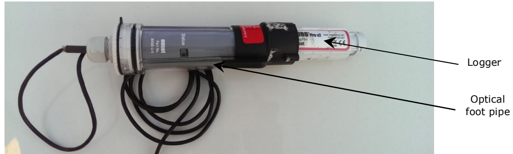
Figure 21: HOBO Pro V2 Relative humidity and ambient temperature sensor and optical pipe
