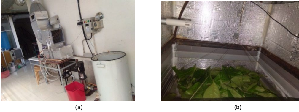
Figure 3: (a) Final assembly of the tea withering testing equipment; (b) Tea commodities in the drying tray, size 36 cm x 36 cm
