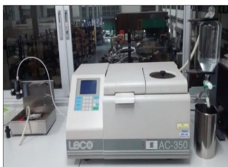
Figure 3: Leco AC-350 bomb calorimeter, Renewable Energy Lab, MTEC
