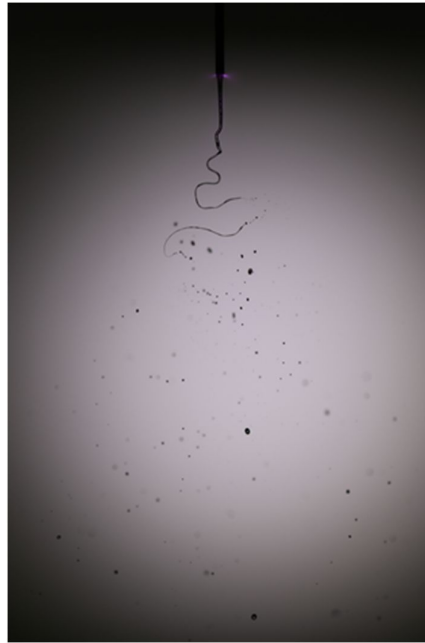
Figure 1: Electro spray mechanism
