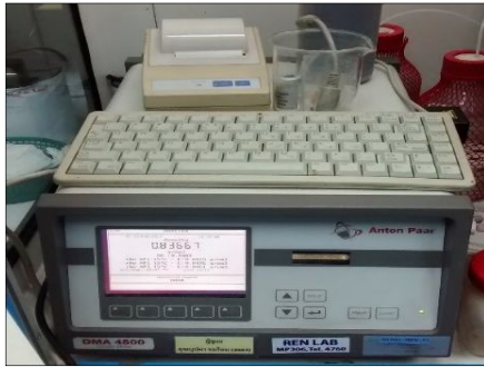
Figure 7: Anton Paar density meter DMA-4500, Renewable Energy Lab, MTEC
