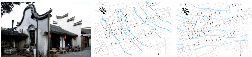
Figure 7: Kuan-Yin Dou and horse-head gable wall (left); summer wind pattern (mid); winter wind pattern (right)
