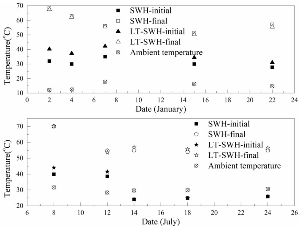
364 Fig.9. Comparison of the initial temperatures and final temperatures in January and July
