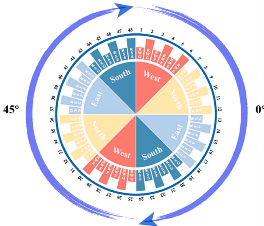
Fig. 9. 48 CFD simulation scenarios for evaluating the impact of different pollutant sources, wind speeds and directions.
