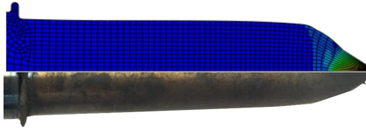
**Figure 7: FE deformation predictions compared to experimental results for aberrant case**
