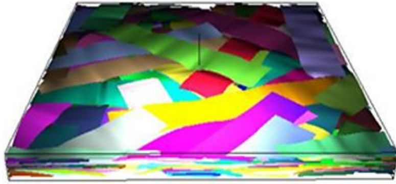
Figure 7: 3D model of DCFP preform from 45 mm long 12K fibre bundles; dimensions: 50 mm × 50 mm × 2 mm.
