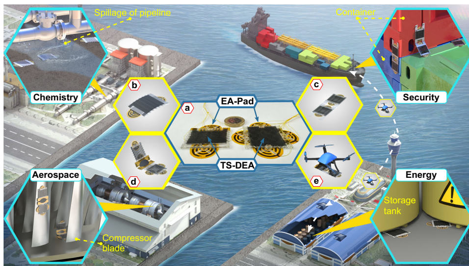
Fig. 8 | Concepts of the Thin-Soft Robots (TS-Robot) for potential applications. a Type-A TS-Robot (left) and Type-B TS-Robot (right), targeting for navigation in narrow gaps on horizontal or vertical surfaces (“Energy” scenario); b Asymmetric configuration of Type-A TS-Robot, targeting for the hybrid solid-liquid environment (“Chemistry” scenario); c Twin Type-A TS-Robot, targeting for transitions
