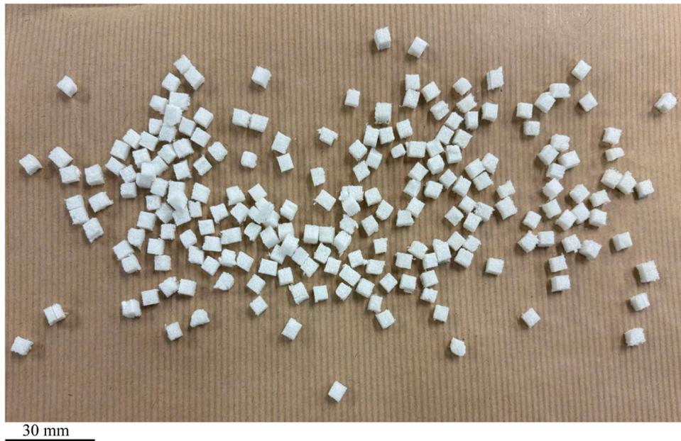
Fig. 1. Illustration of T92.200 foam manually cut into 5 mm cubes for analysis and mixing with asphalt.
