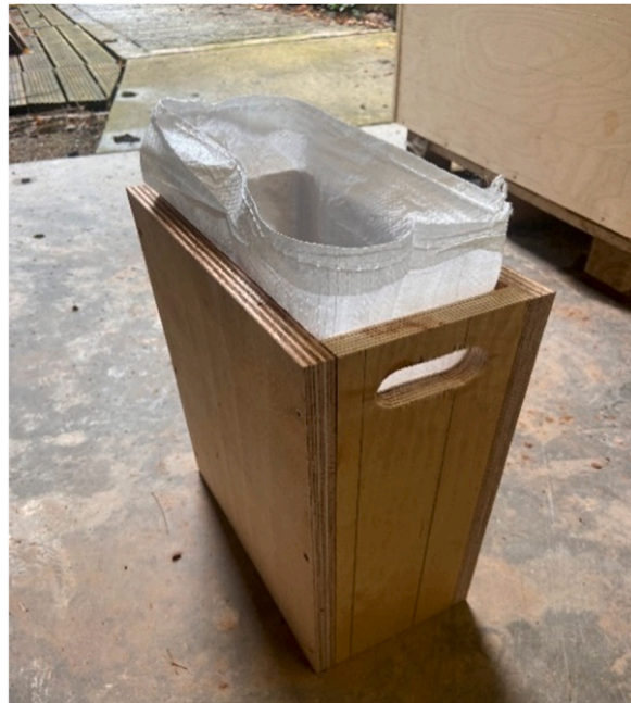
Fig. A. 1. Earthbag block mould.
