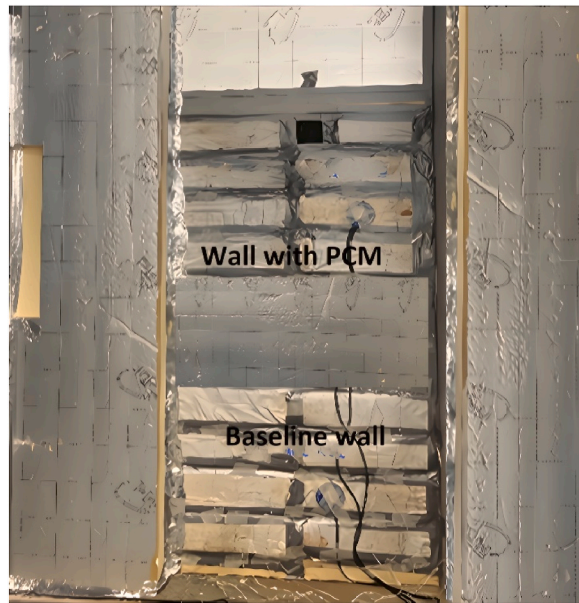
Fig. 3. Tested prototype earthbag wall (with PCM upper and without PCM lower).
