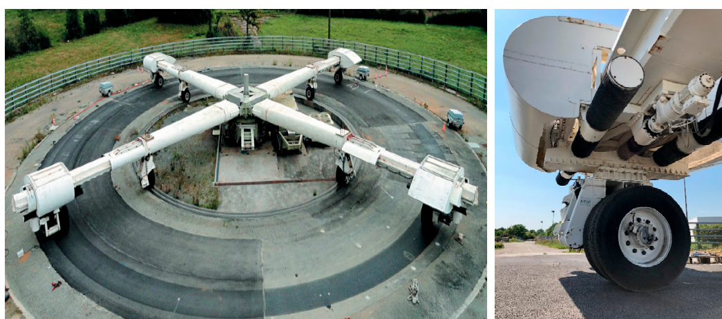
Figure 2. Fatigue carousel for accelerated pavement tests, Nantes—France.
