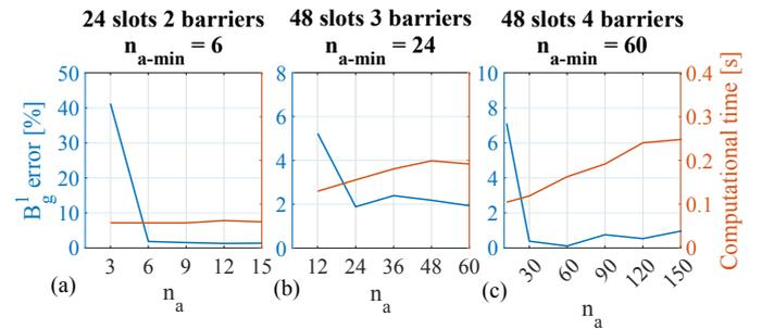
Fig. 9: Error between MEC and FE computation of the first harmonic of  $B_g$  and computational burden as function of the airgap subdivision.
