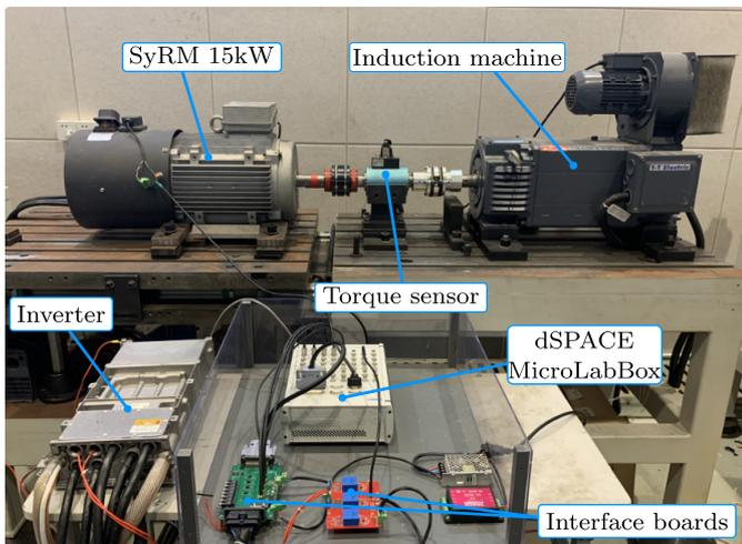
Fig. 18: Experimental setup.
