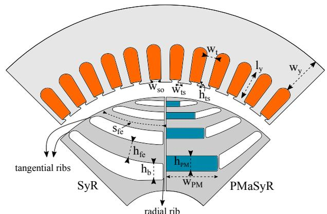
Fig. 1: Stator and rotor geometry parametrization of a typical SyR machine and its PM assisted variant.
