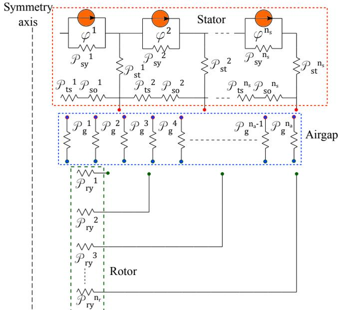
Fig. 3: Magnetic equivalent circuit for the d-axis flux path.
