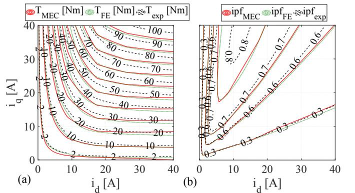
Fig. 21: Comparison between analytically-adjusted, fe and experimental computations of (a) average torque and (b) internal power factor maps.
