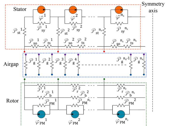
Fig. 4: Magnetic equivalent circuit for the q-axis flux path.
