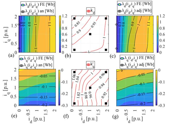
Fig. 16: d-axis and q-axis flux linkages estimation for the 48 slots-3 barriers PMAyR machine: (a,d) analytical and FE computation, (b,e) adjustment factor, (c,f) analytically-adjusted and FE computations.
