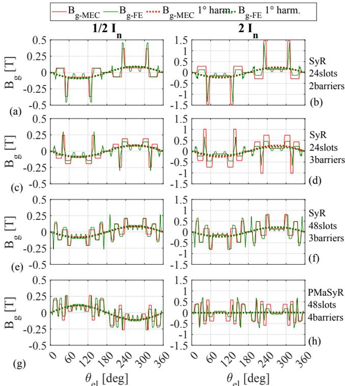
Fig. 8: Analytical and FE airgap flux densities as function of the electrical angle for different machines and q-axis current.
