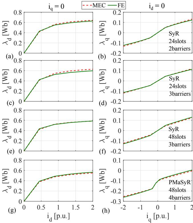
Fig. 10: Comparison between analytical and FE computations of (a) d-axis flux linkage vs current amplitude, (b) q-axis flux linkage vs current amplitude
