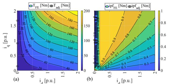
Fig. 17: Comparison between analytically-adjusted and FE computations of (a) average torque and (b) internal power factor maps for the PMAyR machine.
