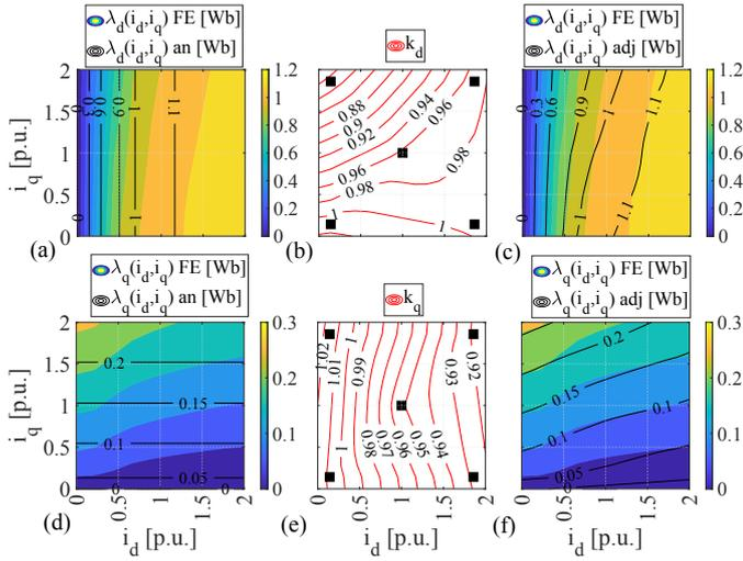
Fig. 13: d-axis and q-axis flux linkages estimation for the 48 slots-3 barriers SyR machine: (a,d) analytical and FE computation, (b,e) adjustment factor, (c,f) analytically-adjusted and FE computations.
