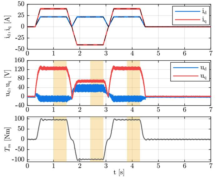
Fig. 19: Example of current and voltage waveforms during the identification with highlighted data log windows.
