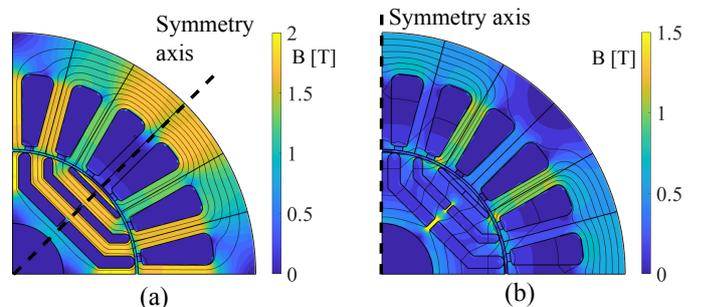
Fig. 2: d-axis (a) and q-axis (b) flux paths.
