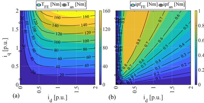
Fig. 11: Comparison between analytical and FE computations of (a) average torque and (b) internal power factor maps considering the 48 slots-3 barriers SyR case.
