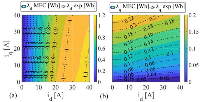
Fig. 20: Comparison between analytically-adjusted and experimental computations of (a) d-axis and (b) q axis flux linkages maps.
