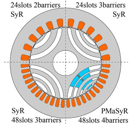
Fig. 6: Machines cross-sections.
