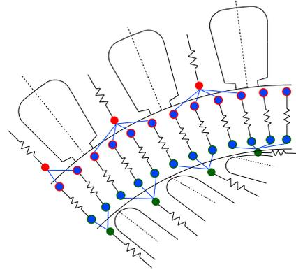
Fig. 5: Circuit modeling of the airgap region.
