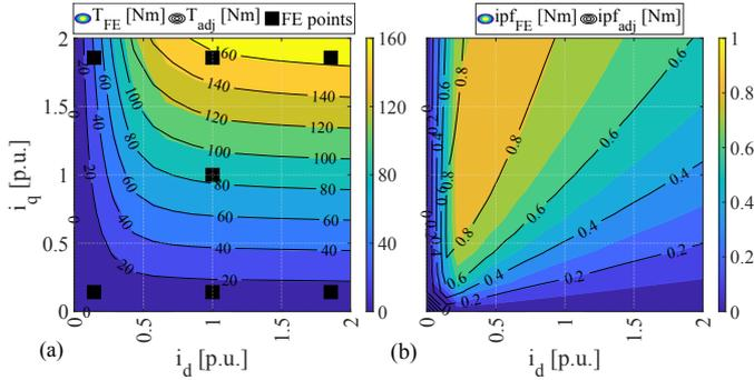
Fig. 15: Comparison between analytically-adjusted and FE computations of (a) average torque and (b) internal power factor maps for the 48 slots-3 barriers SyR machine when the adjustment factors are calculated with 7 static FEAs.
