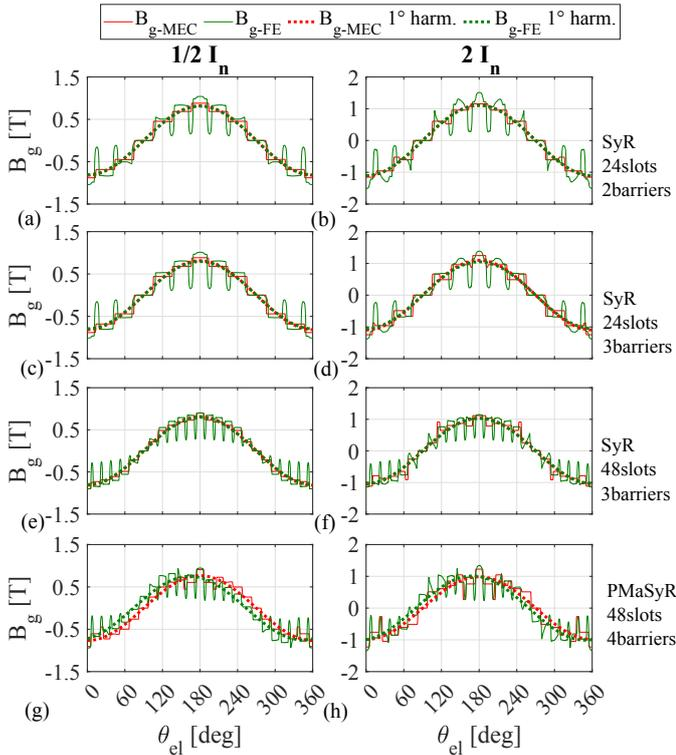
Fig. 7: Analytical and FE airgap flux densities as function of the electrical angle for different machines and d-axis current.
