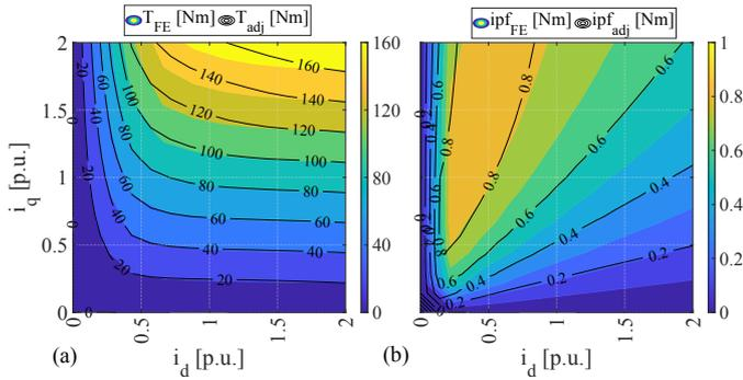
Fig. 14: Comparison between analytically-adjusted and FE computations of (a) average torque and (b) internal power factor maps for the 48 slots-3 barriers SyR machine.
