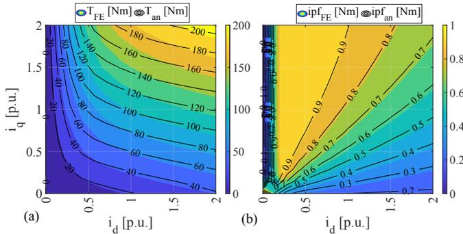
Fig. 12: Comparison between analytical and FE computations of (a) average torque and (b) internal power factor maps of the considered PMAyR machine.
