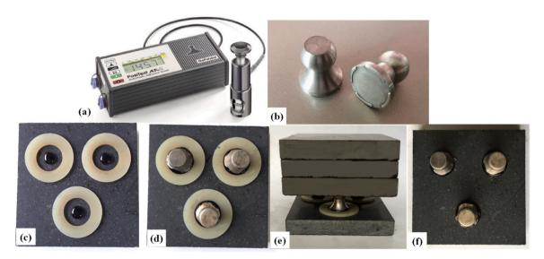
Fig. 3. (a) The Positest AT-A apparatus and (b) stubs, and (c)~(f) sample preparation in the standard BBS test.
