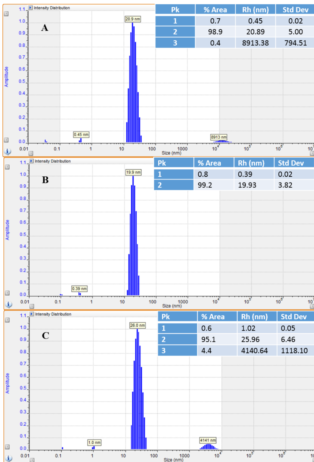
Figure S6: The hydrodynamic radii (Rh) intensity of PEGylated PGA 40% C 18 coated IONPs by DLS. NPs of radius 18 nm were coated with different amount of polymer using interfacial deposition method where (A) 0.05 mg (B) 0.1 mg and (C) 0.2 mg PEGylated PGA 40% C 18 . NP suspension was diluted with ultrapure water to an appropriate concentration to give 300-600 kcps. The Rh of each sample is expressed as the mean particle hydrodynamic radii \pm standard deviation of 10 readings.
