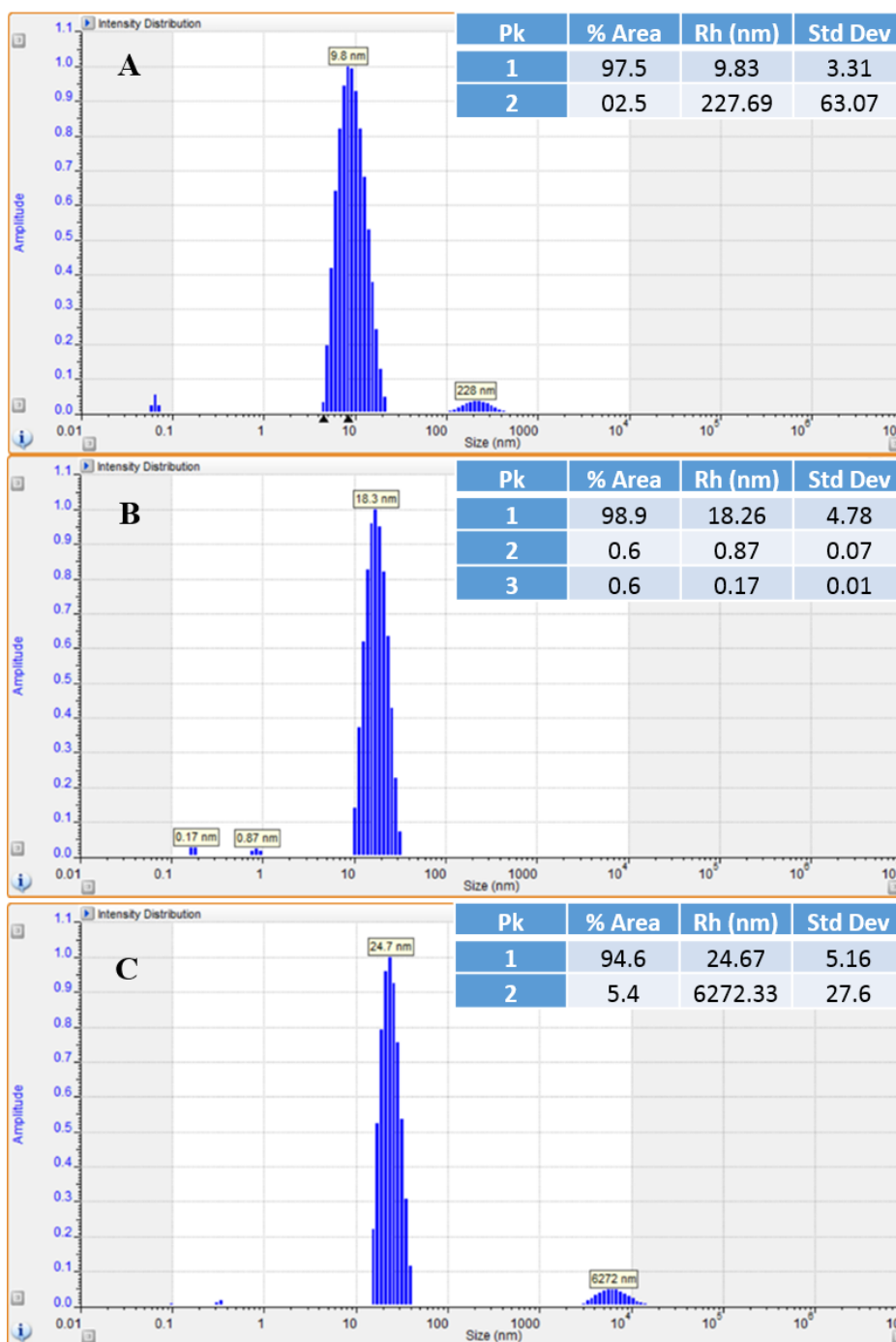
Figure 4: The hydrodynamic radii (Rh) of uncoated IONPs of different size (method 2) by DLS intensity. NPs were prepared by the co-precipitation method at different pH where (A) at pH 0.5, (B) at pH 3 and (C) at pH 4. NP suspension was diluted with ultrapure water to an appropriate concentration to give 300-600 kcps. The Rh of each sample is expressed as the mean particle hydrodynamic radii \pm standard deviation of 10 readings.
