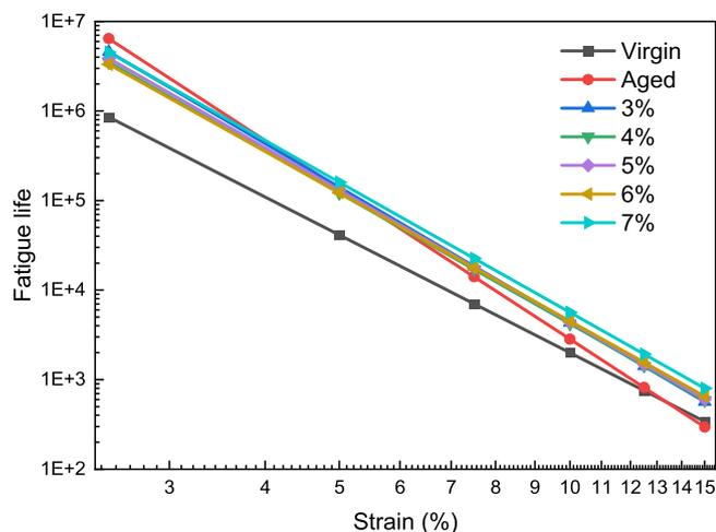
Fig. 7. Correlation between fatigue life and strain.
