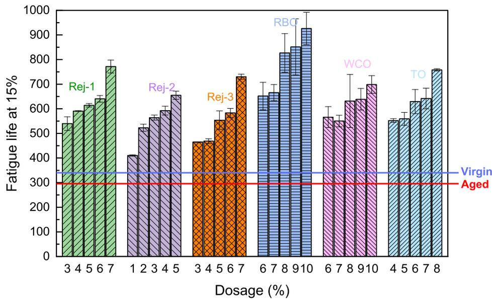
Fig. 5. Fatigue life of binders at strain level of 15 %.
