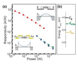
**Figure 4.** a) Photoresponsivity versus incident laser power at T = 300 K and  $\lambda = 633$  nm for planar device geometries based on graphene/InSe/graphene (top) and Au/InSe/Au heterostructures (bottom) ( $V_s = 2$  V and  $V_g = 0$  V). The inset sketches the band alignment for the two heterostructures at  $V_s = 0$  V. b) Work functions ( $\phi$ ) for Au and InSe, and the electron affinity ( $\chi$ ) of graphene.
