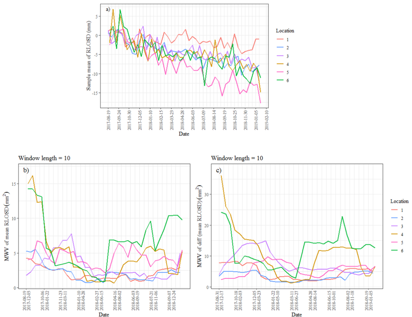
Fig. 3 Spatial trend and moving window variances at six sampling locations. a) Time-series of spatial sample mean of relative LOS displacement (RLOSD). b) Moving window spatial sample variance (MWV) of mean RLOSD. c) Moving window spatial sample variance (MWV) of the detrended mean RLOSD
