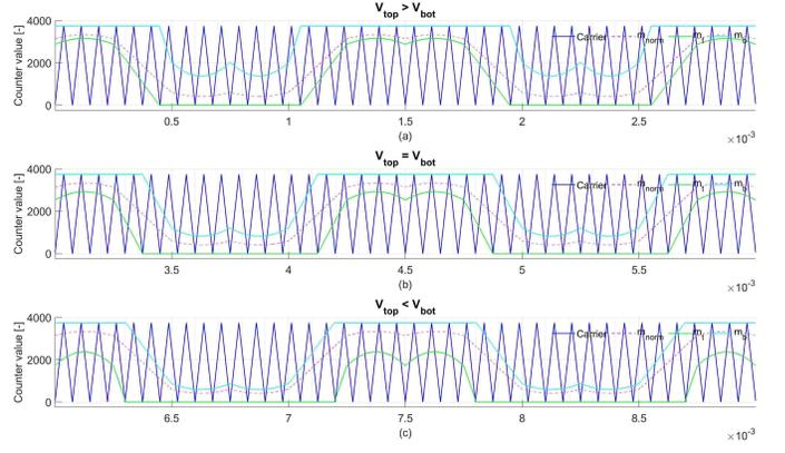
Fig. 6. Equivalent modulation with single-carrier for three typical cases. (a) Case 1:  $V_t > V_b$ . (b) Case 2:  $V_t = V_b$ . (c) Case 3:  $V_t < V_b$ .
