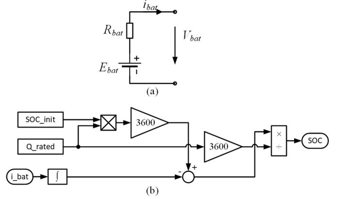
Fig. 2. (a) R-model of battery. (b) Estimation of SOC.
