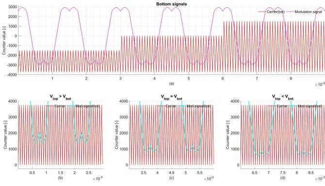
Fig. 5. (a) Bottom signals in classic modulation with two carriers. (b)-(d) Bottom signals in single-carrier modulation. (b) Case 1:  $V_t > V_b$ . (c) Case 2:  $V_t = V_b$ . (d) Case 3:  $V_t < V_b$ .
