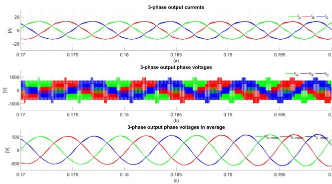
Fig. 10. Simulation results for output voltages and currents. (a) output currents. (b) output voltages. (c) filtered output voltages in average.
