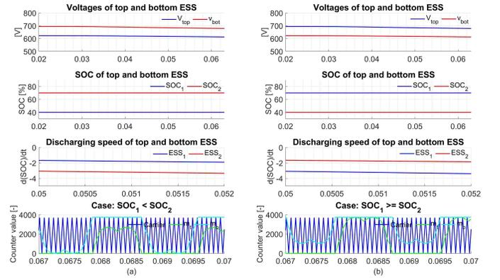
Fig. 8. Simulation results for cases: (a)  $SOC_1 < SOC_2$ . (b)  $SOC_1 \geq SOC_2$ .
