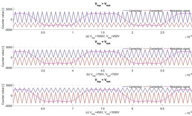
Fig. 3. Classic double-carrier modulation. (a) Case 1:  $V_t > V_b$ . (b) Case 2:  $V_t = V_b$ . (c) Case 3:  $V_t < V_b$ .
