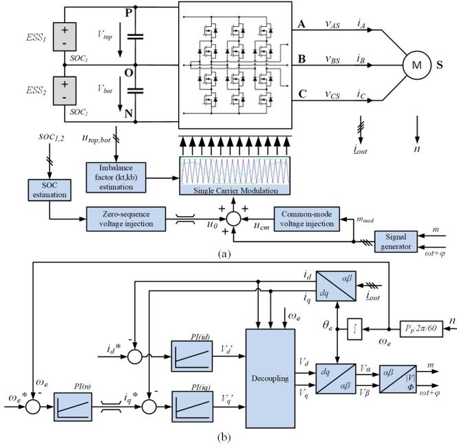
Fig. 7. Block diagram of the proposed control method: (a) Modified single-carrier modulation. (b) Closed cascade control loops of PMSM drive.
