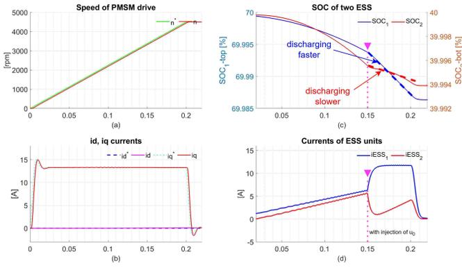
Fig. 9. Simulation results for performance of PMSM drive: (a) machine speed. (b)  $i_d$  and  $i_q$  currents. (c) SOC of ESS units. (d) Currents of ESS units.
