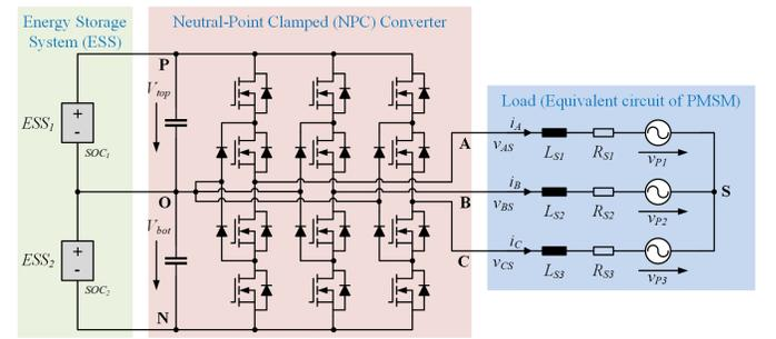
Fig. 1. System topology of the three-phase three-level NPC converter-fed PMSM drive.
