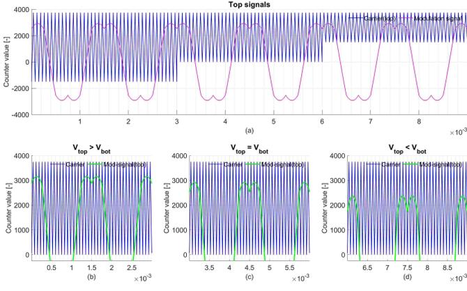
Fig. 4. (a) Top signals in classic modulation with two carriers. (b)-(d) Top signals in single-carrier modulation. (b) Case 1:  $V_t > V_b$ . (c) Case 2:  $V_t = V_b$ . (d) Case 3:  $V_t < V_b$ .
