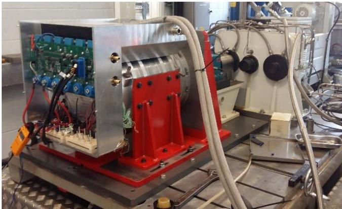
Fig. 21 Prototype of rare-earth-free machine.
