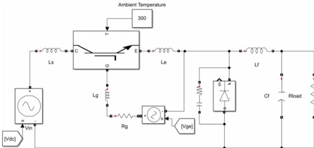
Fig. 11. Simulink implementation of a buck converter using the proposed model as the switching device.
