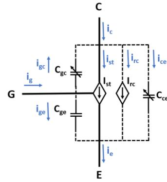
Fig. 6. IGBT equivalent circuit.
