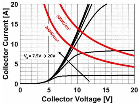
Fig. 2. TCAD results for static  $I_c$ - $V_{ce}$  characteristics of the IGBT at different gate voltages.
