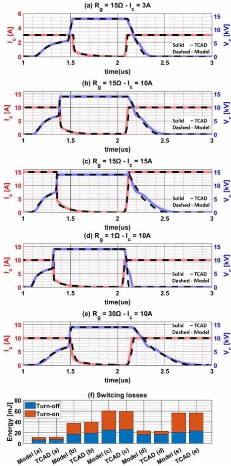
Fig. 8. Switching behaviour comparison between the proposed model and TCAD simulation results.
