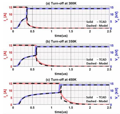
Fig. 10. Inductive turn-off process comparison between the TCAD and behavioural model results at temperatures 300-450K.
