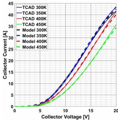
Fig. 5. Comparison between TCAD and behavioural model  $I_c$ - $V_{ce}$  characteristics at different temperatures for  $V_{ge} = 15V$ .
