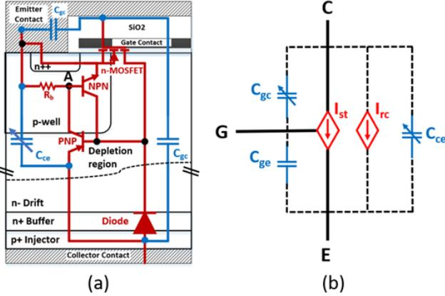
Fig. 1. (a) IGBT cell structure and internal parasitic components representation, (b) IGBT compact model.
