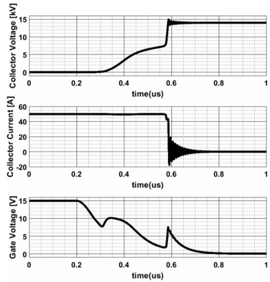
Fig. 12. IGBT waveforms during the buck converter operation.
