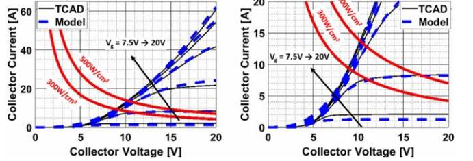
Fig. 3. Comparison between TCAD and behavioural model  $I_c$ - $V_{ce}$  characteristics under different gate voltages.
