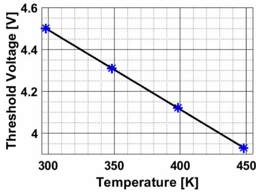
Fig. 4. Temperature dependence of the gate threshold voltage.
