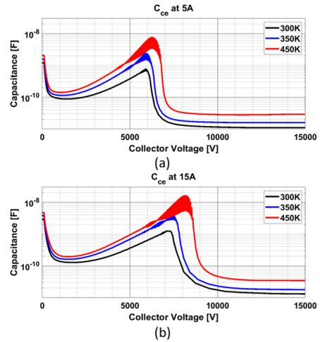
Fig. 9. Temperature dependence of the  $C_{ce}$  at collector current of (a) 5A and (b) 15A.
