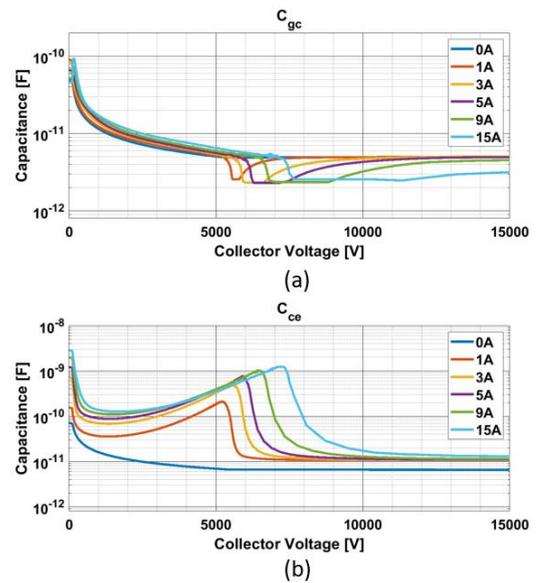
Fig. 7. Voltage and current dependence of the (a)  $C_{gc}$  and (b)  $C_{ce}$ .
