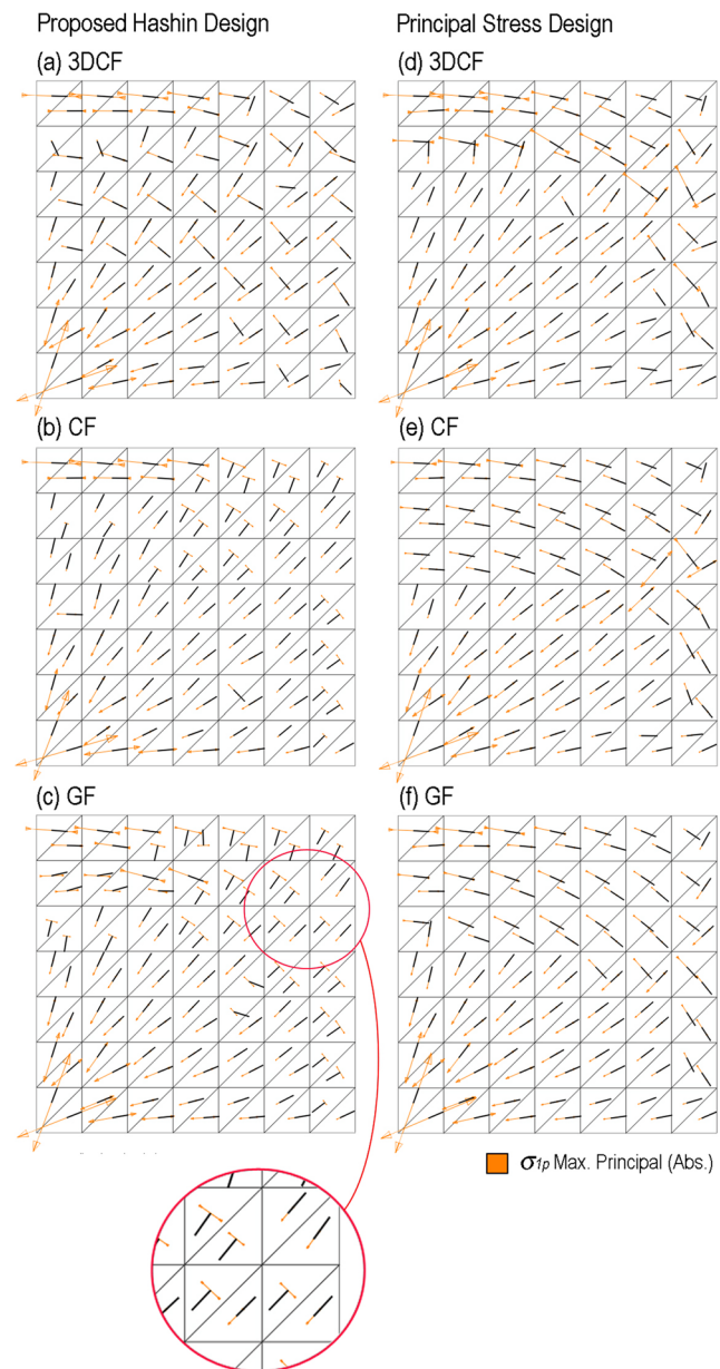
Fig. 3 Problem 1: final designs obtained by the here proposed HA-OCM, (a) to (c), and principal stress design, (d) to (f). Orange arrows are maximum principal stresses in absolute \sigma_{1p} . Black lines are local material 1-directions (fibre). In (g), the red circle highlights the occurrence of material oriented at 0^\circ and 90^\circ with the principal stress direction at the optimised design, a possible result in HA-OCM
