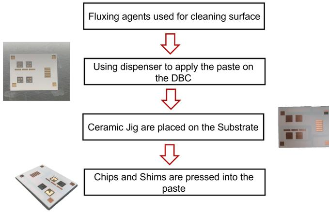
Fig. 10: Assembly flowchart
