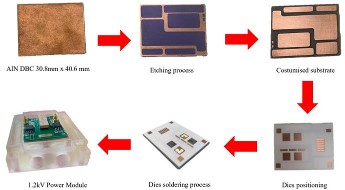
Fig. 9: Assembly flowchart
