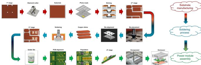
Fig. 8: Manufacturing process
