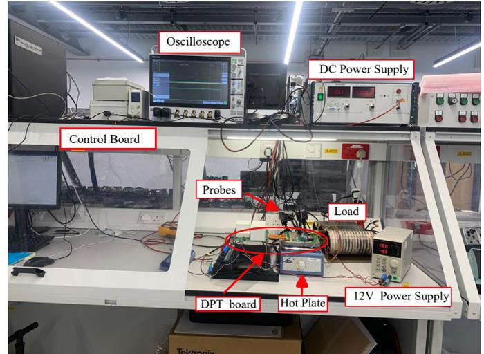
Fig. 12: Double Pulse Test board
