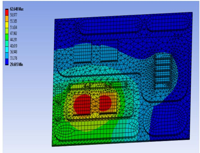
Fig. 7: FE thermal simulation
