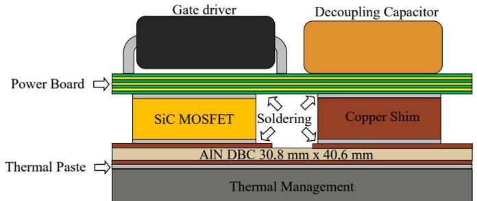
Fig. 2: Cross-sectional view
