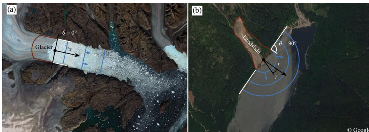
Figure 1. Landslide-tsunami settings represented by idealised geometries: (a) Helheim Glacier representing a 2D geometry (contains modified Copernicus Sentinel data, 2016, processed by Pierre Markuse) and (b) 2007 Chehalis lake case representing a 3D geometry (adapted from Google maps).
