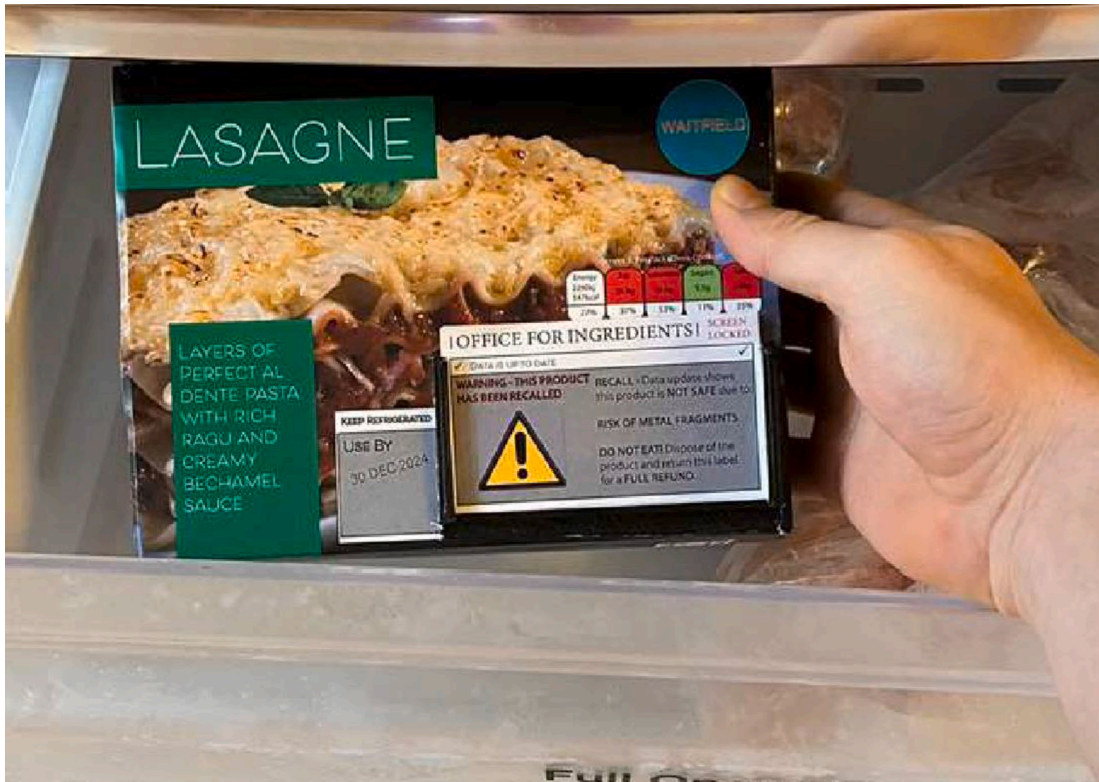
Fig. 7. The packaging displays a range of information 'live', updated via the internet from the data trust. The label cycles through different screens providing a range of information about the food.
