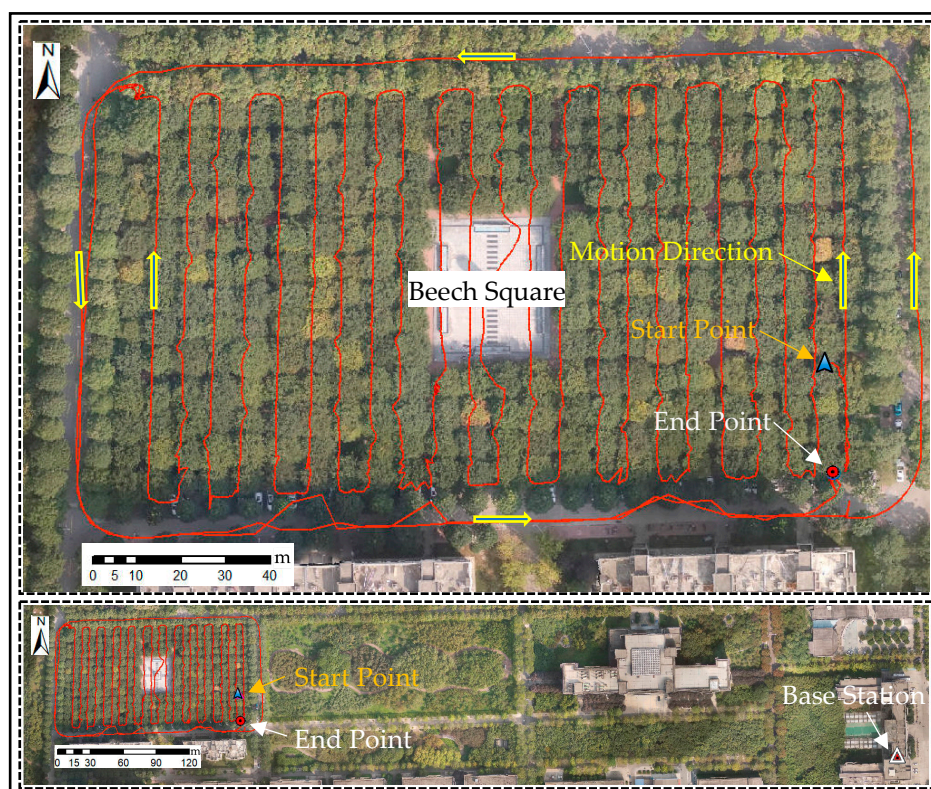
Figure 12. The trajectory of the kinematic GNSS receiver's carrier under forest scene.
