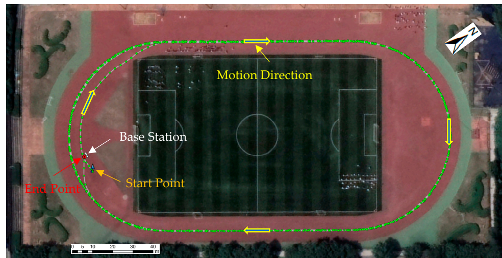
Figure 1. The trajectory of the kinematic GNSS receiver's carrier under an open environment.
