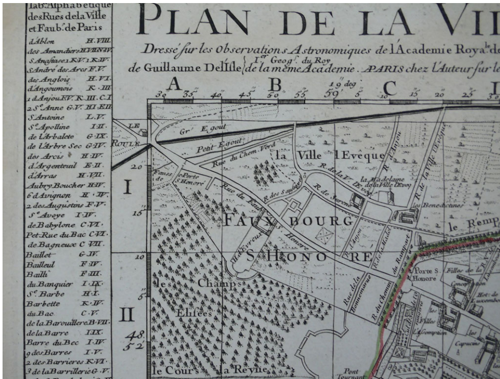
Figure 3. Detail of the graticule divisions on Delisle's 1716 map of Paris, with 15 seconds of latitude on the meridian lines and 20 seconds of longitude on the parallel lines. Source: David Rumsey Map Collection, List No. 4764.018, reproduced with permission.
