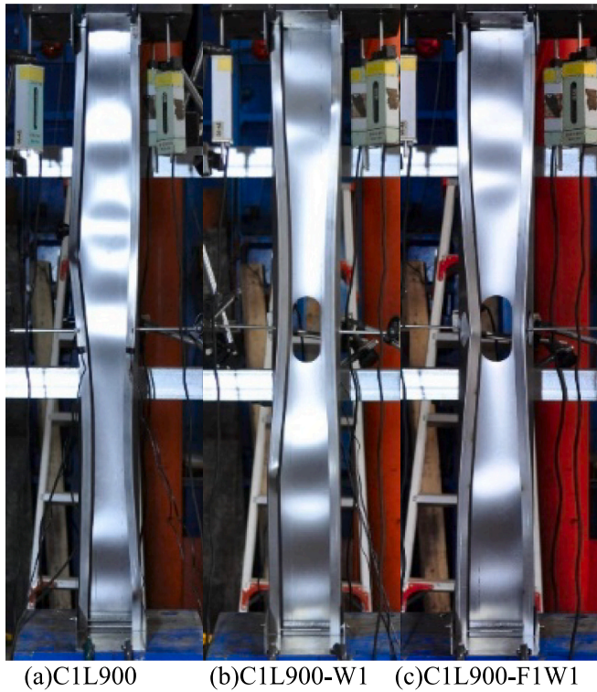
Fig. 10. Failure modes of C1-section specimens with a length of 900 mm.
