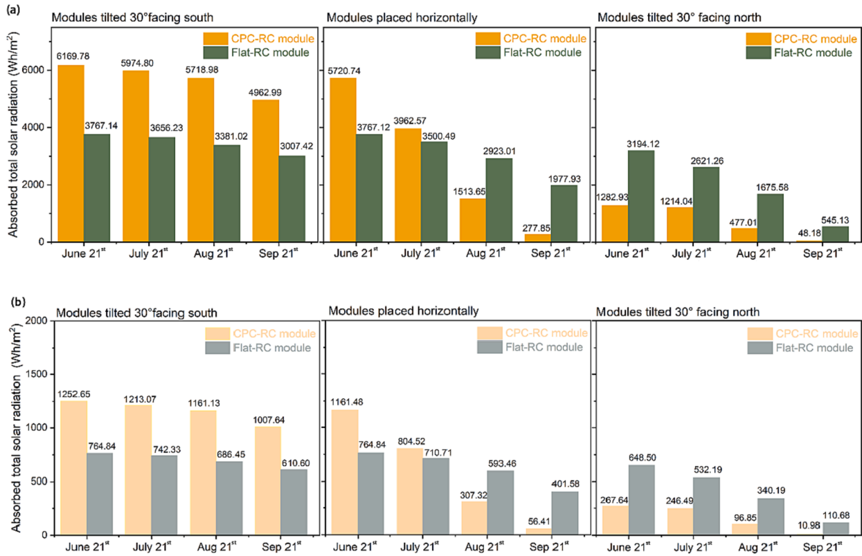
Fig. 12. Total solar radiation absorbed by the CPC-RC and flat-RC modules at three placements on four typical days. (a) Black-painted RC emitter (b) Metamaterial-covered RC emitter.
