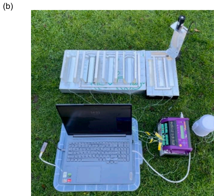
Fig. 7. (a) Schematic of the RC experimental system. (b) In-situ experimental setup of the RC system. The experimental system is located in the open field at the University of Nottingham (52.94°N, 1.09°W), UK with the site altitude being 60 m.
