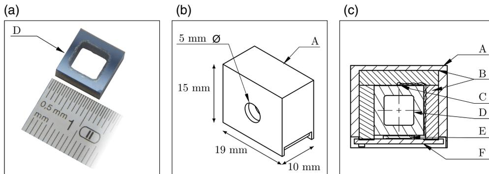
**Fig. 2** Design of cesium MEMS cell and heating assembly. (a) Photograph of cesium MEMS cell with 3 mm optical path. (b) Drawing of the external cell oven assembly. (c) Cross-section of oven, insulation and cell. A: 3D printed cell housing, B: calcium-magnesium silicate thermal insulation, C: t-type thermocouple, D: cesium 3 mm MEMS cell, E: non-inductive SMD resistor, F: heater interface PCB.
