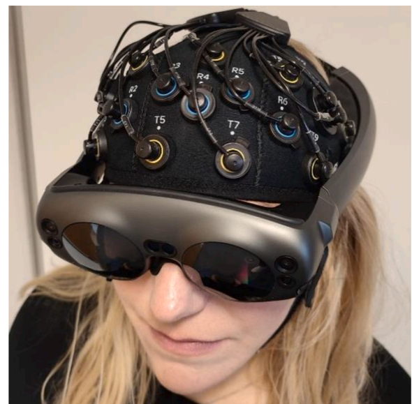
Fig. 4. User wearing Artinis Brite23 fNIRS device together with Magic Leap AR Glasses.
