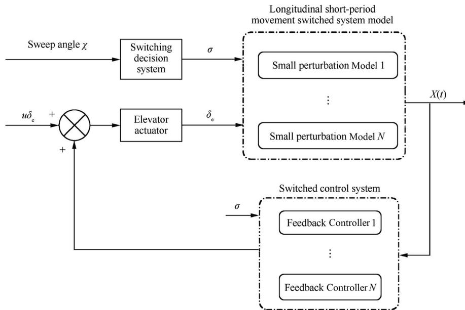
Fig. 2 Structure of switched control system (reproduced from Ref. 16).
