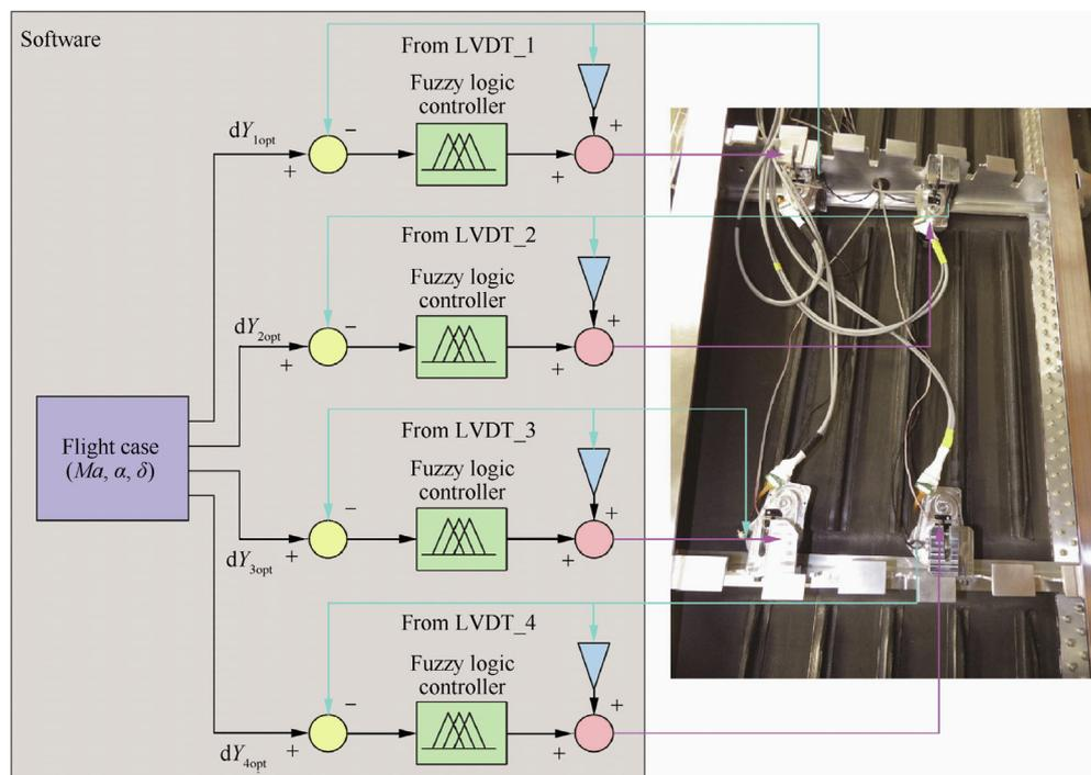
Fig. 5 Open-loop control architecture of morphing wing model.<sup>91</sup>
