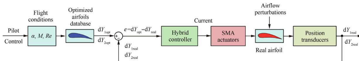
Fig. 7 Block diagram of controlled morphing wing system Ref. 111.
