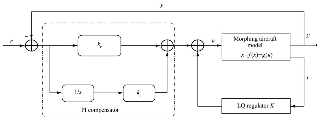
Fig. 3 Robust controller's structure (reproduced from Ref. 29).
