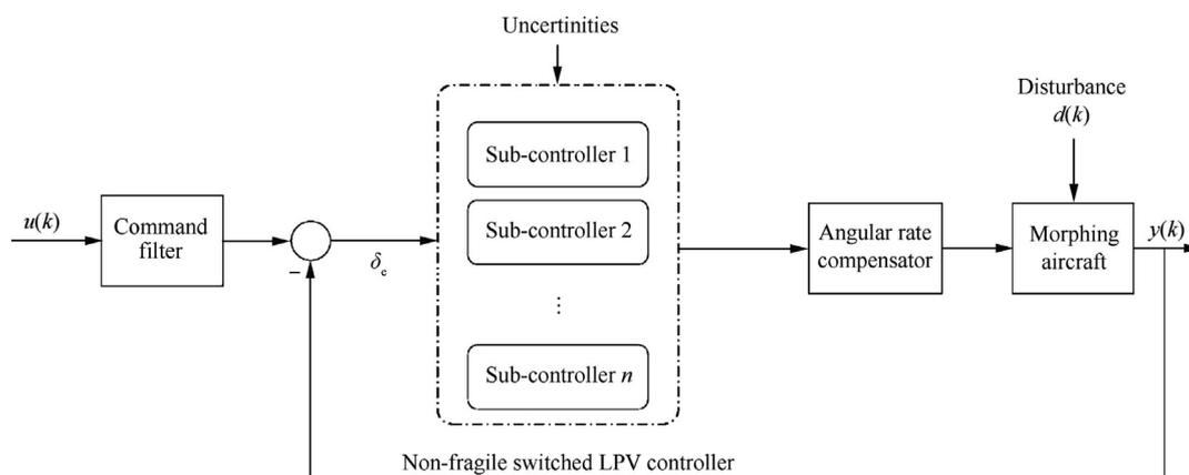
Fig. 4 Structure diagram of flight control system (reproduced from Ref. 34).
