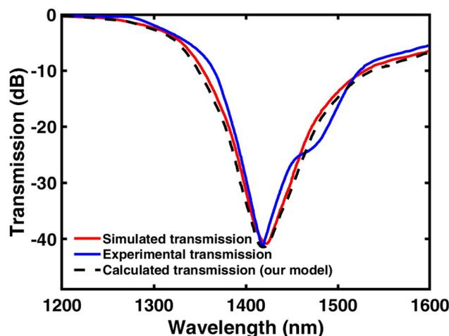
Fig. 2 The measured (blue line) [25] and calculated theoretically (red line) transmissions through D-shaped optical fiber [25] with 8.2 μm core diameter, 125 μm cladding diameter and 0.092 μm ITO thickness layer. The dashed black line represents the calculated transmission based on utilized model in our numerical simulations
