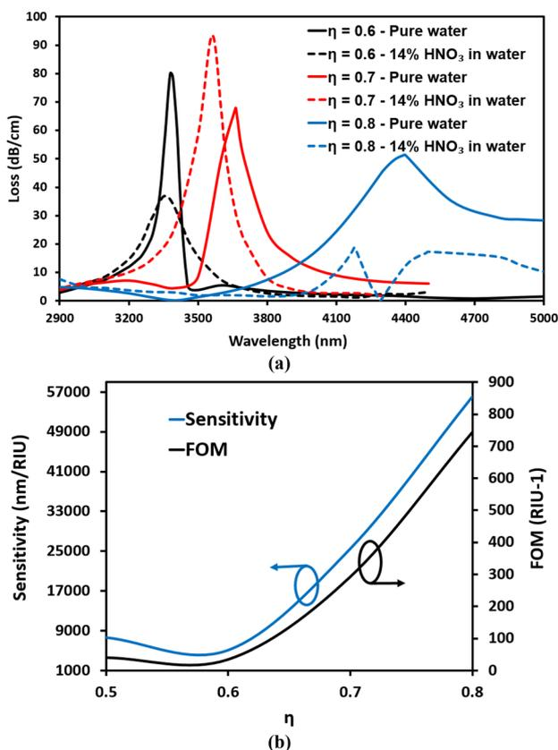
**Fig. 8** **a** Wavelength dependent optical loss of core mode at different values of  $\eta$ , and **b** the sensitivity ( $S$ ) and FOM at different values of  $\eta$ . The initial dimensions of  $w_g = 0.4 \mu\text{m}$  and  $h = 5 \mu\text{m}$  were used (see Fig. 1b).  $t_g$  was fixed at its optimized value of  $50 \text{ nm}$
