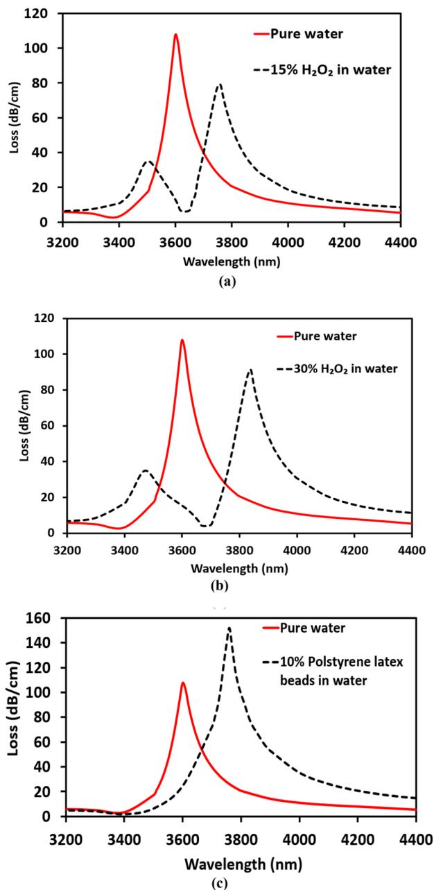
**Fig. 13** Confinement optical loss spectra of the core mode of the geometrically optimized (Table 1) D-shaped InF<sub>3</sub>-based glass optical fiber SPR sensor for pure water and **a** dissolved 15% v/v H<sub>2</sub>O<sub>2</sub> in water, **b** dissolved 30% v/v H<sub>2</sub>O<sub>2</sub> in water, **c** suspended 10% v/v polystyrene 0.1 μm diameter beads in water
