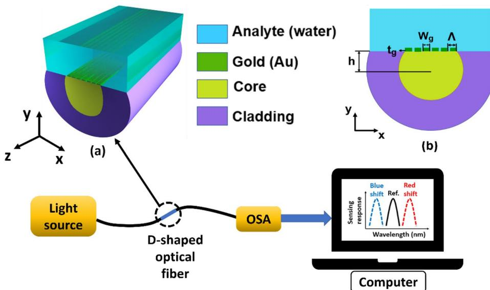
resin to avoid fiber fracture, as fluoride glasses exhibit a low Young’s modulus and hardness compared to silica glass. To fabricate the Au grating, first, an Au layer can be deposited on the polished surface of the D-shaped InF<sub>3</sub>-based glass fiber via thermal evaporation, magnetron sputtering, or pulsed laser deposition [23] and then the grating patterned into the deposited Au coating using nanolithography [23].
