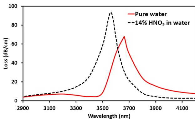
**Fig. 6** Confinement optical loss spectra of the core mode for both pure water and 14%  $v/v$   $\text{HNO}_3$  in water. The dimensions of the Au grating in the D-shaped  $\text{InF}_3$ -based glass optical fiber SPR optical sensor are  $t_g = 50$  nm,  $w_g = 0.4$   $\mu\text{m}$ ,  $\eta = 0.7$ , and  $h = 5$   $\mu\text{m}$  (see Fig. 1b)
