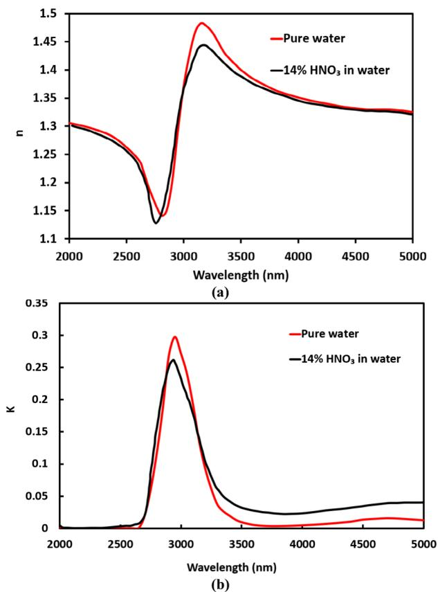
**Fig. 3** **a** Real and **b** imaginary parts (*i.e.*, the extinction coefficient), of the refractive index of pure water and 14% $v/v$  HNO<sub>3</sub> polluted water due to fundamental vibrations of O–H of water at  $\sim 3 \mu\text{m}$  wavelength [47, 48]
