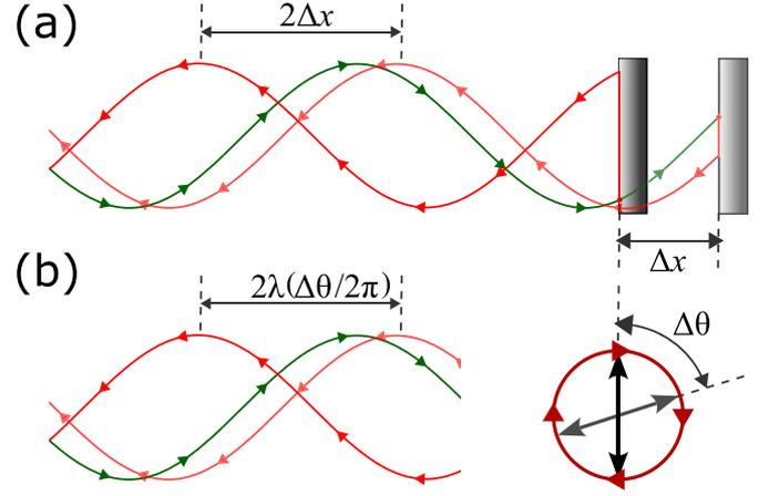
**Figure 2.** (a) Michelson interferometer phase from mirror motion. (b) Comparable effect from rotating a reflecting dipole to interact with a delayed polarisation component.
