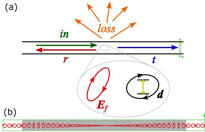
**Figure 1.** (a) Schematic cartoon of the scattering process. The input is split between reflection, transmission and loss, with the coefficients determined by the waveguide electric field at the location of the TLS (red), and the transition dipole of the TLS (black). (b) Polarisation structure in a simple waveguide, consisting of a high-index rectangular block (grey) in air (white). Polarisation ellipses are shown through a cut, with light propagating up the page (frame arrow).
