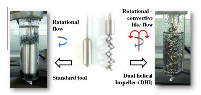
Fig. 3. The idea through comparison between the impellers and the generated flows during rotation.
