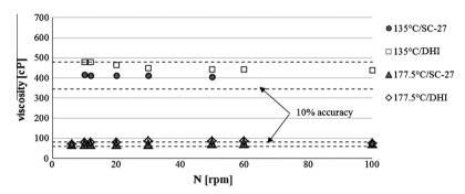
**Fig. 9.** Viscosity measurements by using LV on a 40/60 bitumen at T = 135 °C and 177.5 °C.
