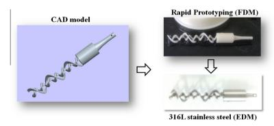
Fig. 6. DHI manufacturing process: design, rapid prototyping through FDM and final tool produced with EDM.
