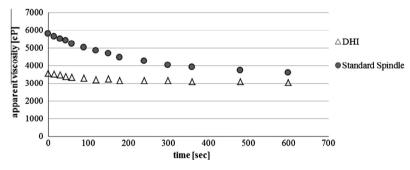
**Fig. 10.** Apparent viscosity of a TR-MB at 177.5 °C by using LV viscometer at 12 rpm.
