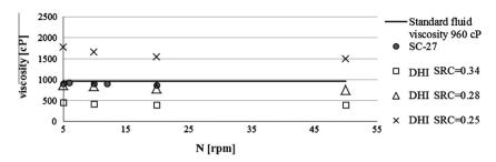
Fig. 8. Viscosity measurements by using LV on standard fluid 960.
