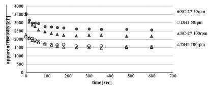
**Fig. 11.** Apparent viscosity of a TR-MB at 177.5  $^{\circ}$ C by using HA viscometer at 50–100 rpm.
