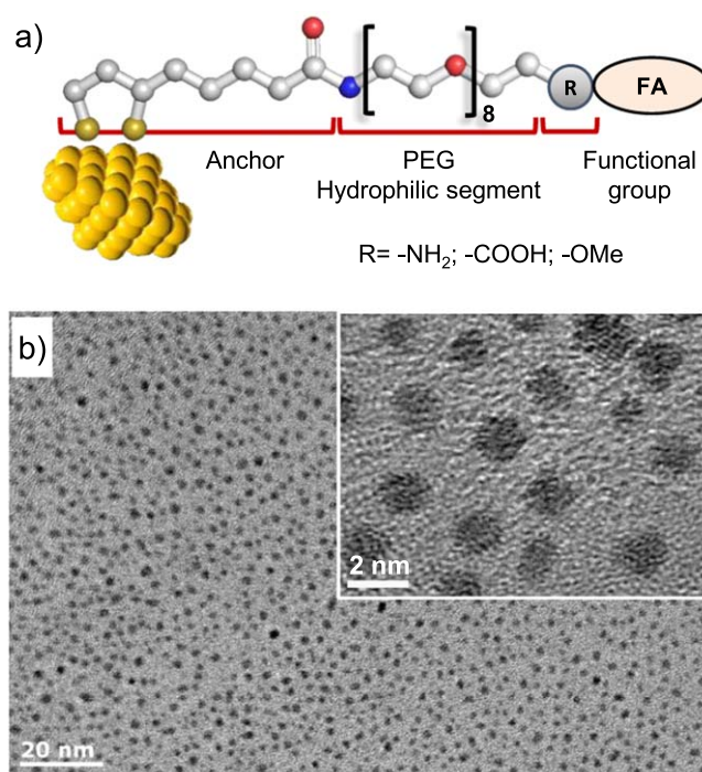
Figure 1. (a) Cartoon of an Au nanocluster capped with DHLA-PEG ligands terminated with different functional groups. (b) TEM and HR TEM images of Au NC capped with LA-PEG 200 -based ligands with NH_2 functional ending group.
