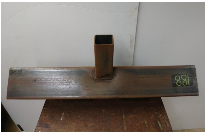
(b) Test vs FE comparison for chord crown failure (C) mode of SBB T-joint (T-80×80×4-140×140×4×45°).
