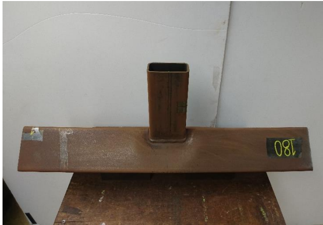
(a) Test vs FE comparison for chord crown failure (C) mode of SBB T-joint (T-50×100×4-120×120×3×45°).
