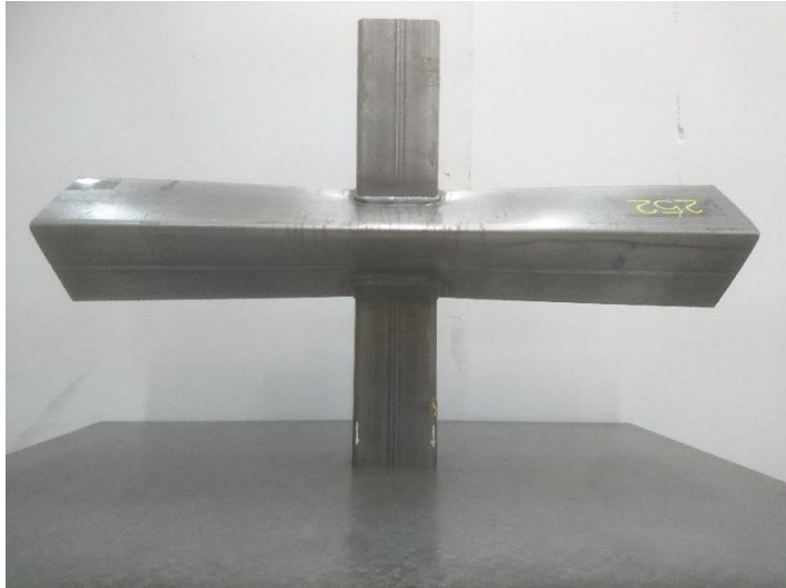
(b) Test vs FE comparison for chord crown failure (C) mode of SBB X-joint (X-50×100×4-120×120×3×45°).
