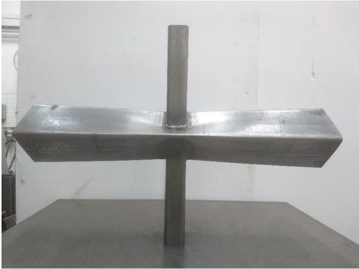
(a) Test vs FE comparison for chord crown failure (C) mode of SBB X-joint (X-100×50×4-120×120×3×45°).
