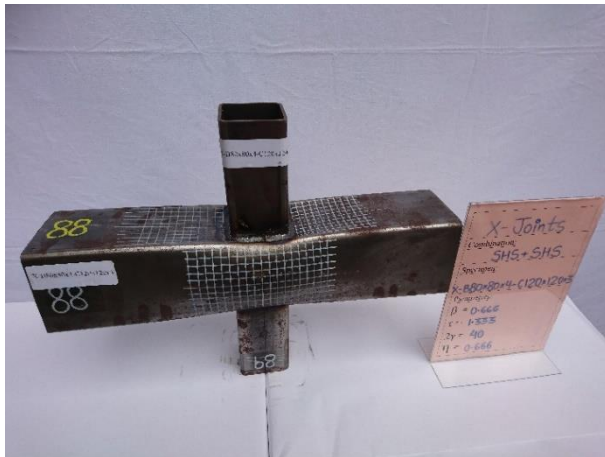
(a) Test vs FE comparison for RHS X-joint failed by F mode at room temperature.
