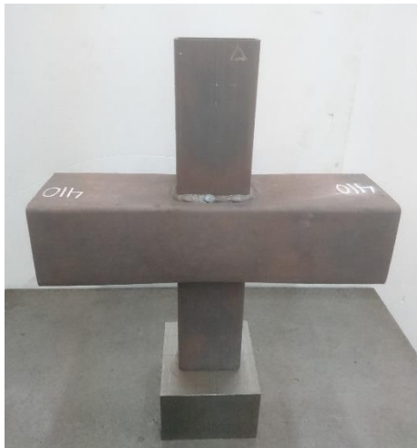
(a) Test vs FE comparison for RHS X-joint failed by F mode for post-fire condition.
