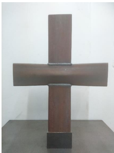
(b) Test vs FE comparison for RHS X-joint failed by S mode for post-fire condition.
