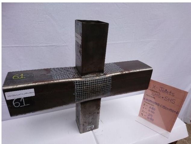
(b) Test vs FE comparison for RHS X-joint failed by F+S mode at room temperature.
