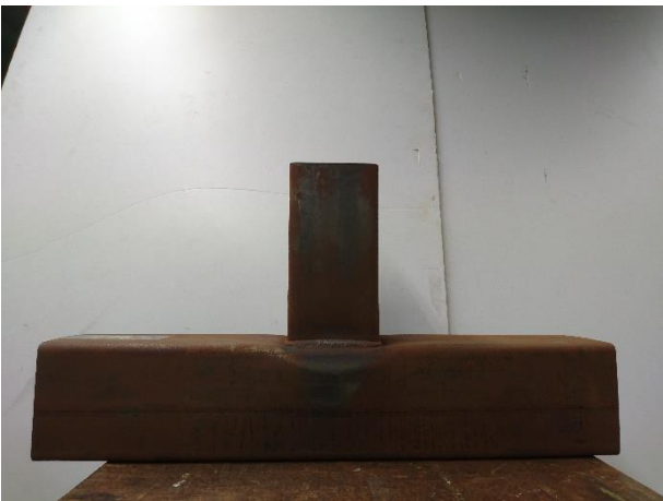
(b) Test vs FE comparison for RHS T-joint failed by F+S mode at ambient temperature.
