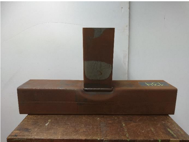
(c) Test vs FE comparison for RHS T-joint failed by S mode at ambient temperature.
