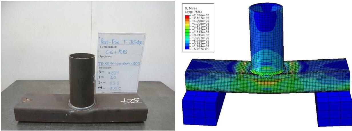
(a) Test vs FE comparison for CHS-to-RHS T-joint failed by F mode for post-fire conditions.
