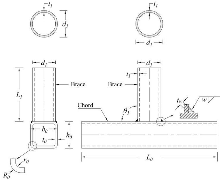
Fig. 1. Representations of geometric notations for CHS-to-RHS T-joint (also valid for X-joint).
