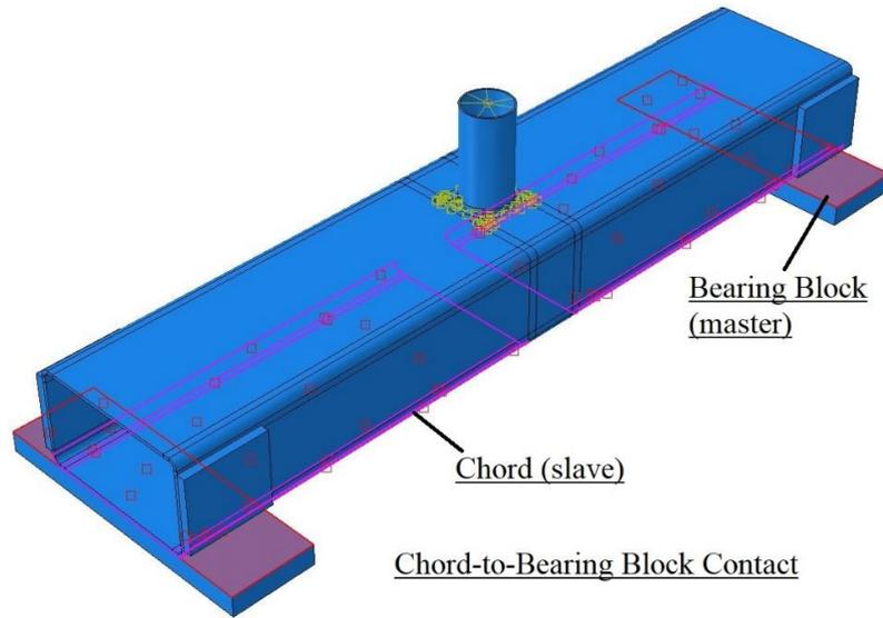
(b) Chord-to-bearing block contact interaction in CHS-to-RHS T-joint.
