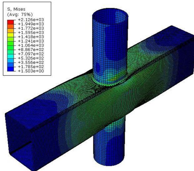
(b) CHS-to-RHS X-joint failed by F+S mode at elevated temperature.
