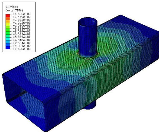
(a) CHS-to-RHS X-joint failed by F mode at elevated temperature.
