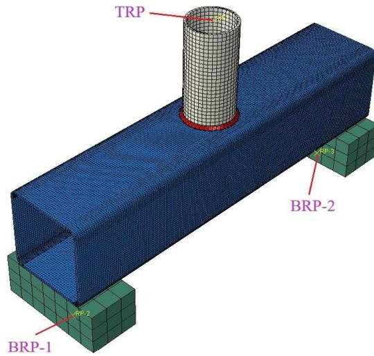
(a) Typical FE model of CHS-to-RHS T-joint with small  $\beta$  value ( $\beta=0.59$ ).
