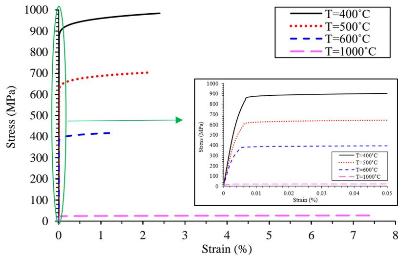
Fig. 14. Stress-strain curves at elevated temperatures [53].
