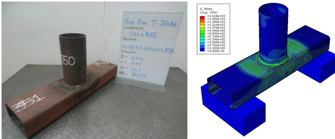
(b) Test vs FE comparison for CHS-to-RHS T-joint failed by F+S mode for post-fire conditions.
