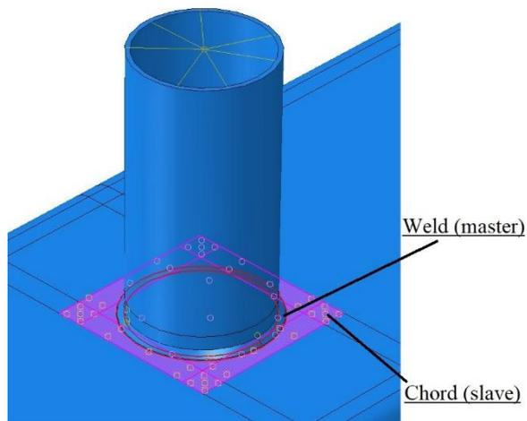
(b) Weld-to-chord tie connection in CHS-to-RHS T- and X-joints.
