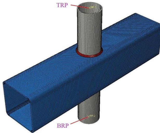
(a) Typical FE model of CHS-to-RHS X-joint with small  $\beta$  value ( $\beta=0.59$ ).
