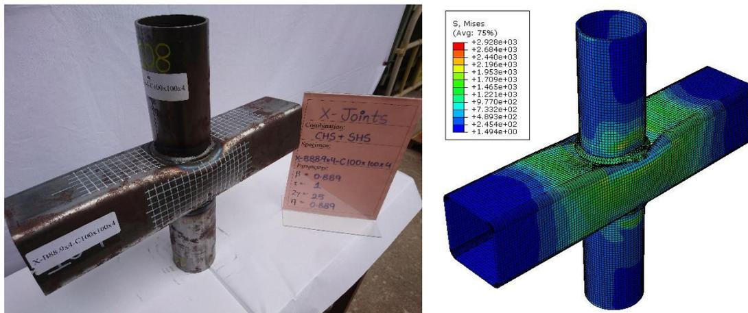
(b) Test vs FE comparison for CHS-to-RHS X-joint failed by F+S mode at ambient temperature.
