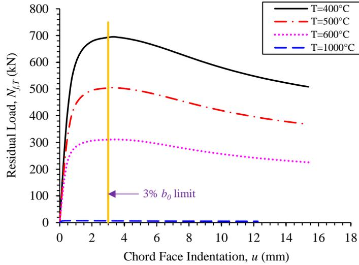
(b) Variations of load vs deformation curves for typical CHS-to-RHS X-joint ( $X-90\times 6-100\times 100\times 6$ ;  $\beta=0.90$ ) failed by F+S mode at elevated temperatures.
