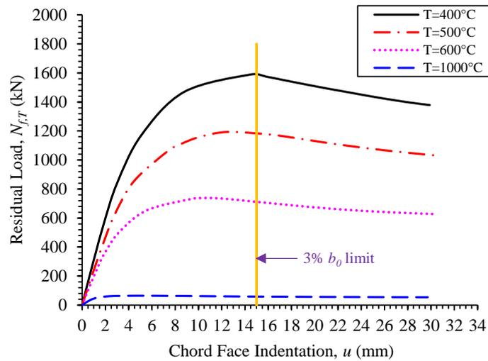
(b) Variations of load vs deformation curves for typical CHS-to-RHS T-joint (T-450×10-500×500×10;  $\beta=0.90$ ) failed by F+S mode at elevated temperatures.
