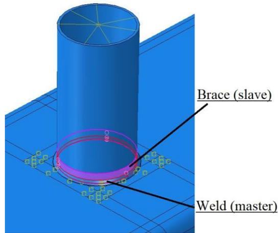
(a) Weld-to-brace tie connection in CHS-to-RHS T- and X-joints.
