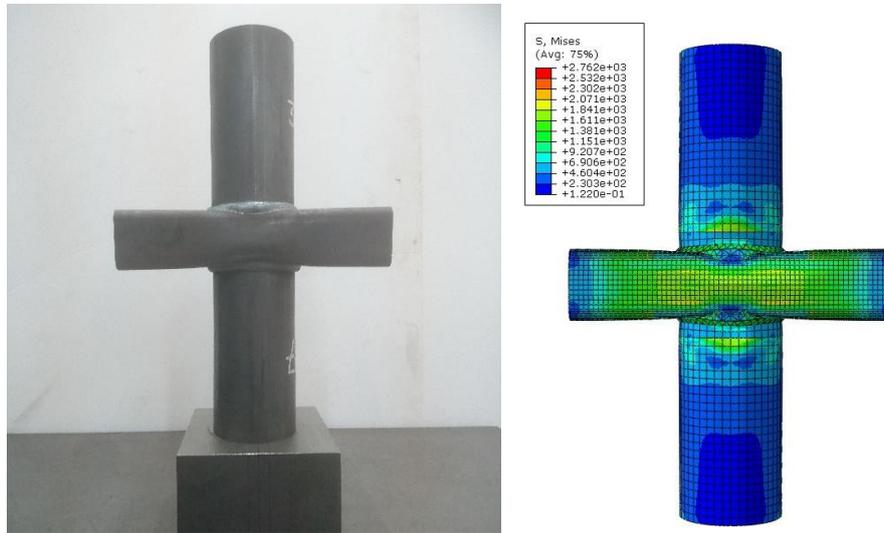
(b) Test vs FE comparison for CHS-to-RHS X-joint failed by F+S mode for post-fire conditions.
