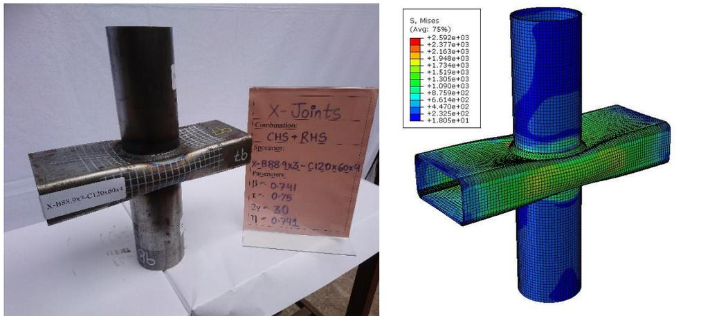
(a) Test vs FE comparison for CHS-to-RHS X-joint failed by F mode at ambient temperature.
