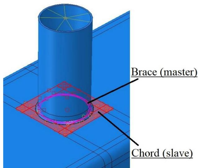
(a) Brace-to-chord contact interaction in CHS-to-RHS T- and X-joints.
