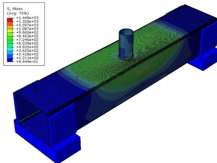
(a) CHS-to-RHS T-joint failed by F mode at elevated temperature.
