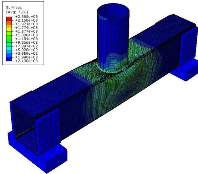
(b) CHS-to-RHS T-joint failed by F+S mode at elevated temperature.
