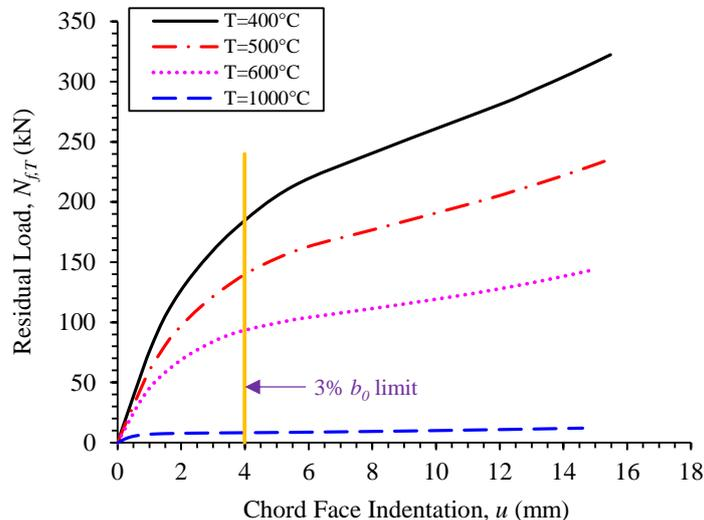
(a) Variations of load vs deformation curves for typical CHS-to-RHS X-joint (X-40×4-133×240×8;
