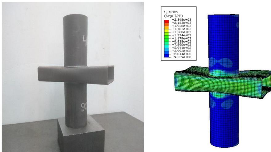
(a) Test vs FE comparison for CHS-to-RHS X-joint failed by F mode for post-fire conditions.
