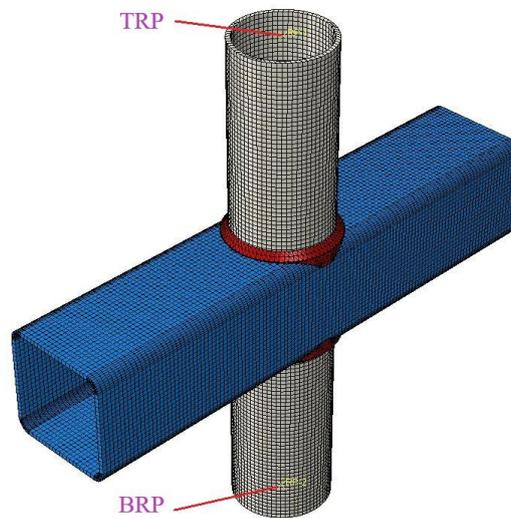
(b) Typical FE model of CHS-to-RHS X-joint with large  $\beta$  value ( $\beta=0.89$ ).
