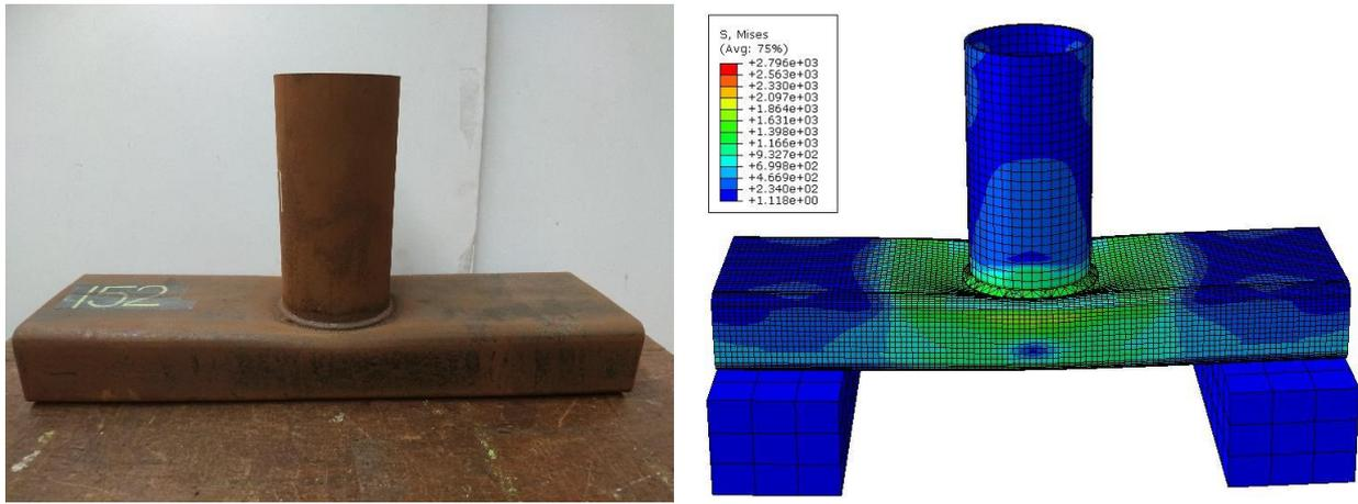
(b) Test vs FE comparison for CHS-to-RHS T-joint failed by F+S mode at ambient temperature.
