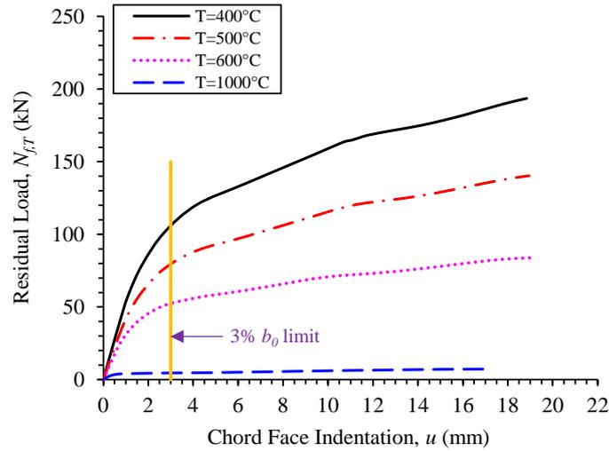
(a) Variations of load vs deformation curves for typical CHS-to-RHS T-joint (T-30×3-100×100×6;  $\beta=0.30$ ) failed by F mode at elevated temperatures.
