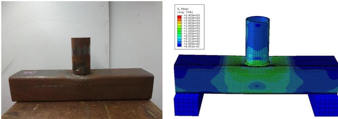
(a) Test vs FE comparison for CHS-to-RHS T-joint failed by F mode at ambient temperature.
