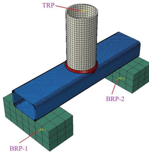
(b) Typical FE model of CHS-to-RHS T-joint with large  $\beta$  value ( $\beta=0.89$ ).
