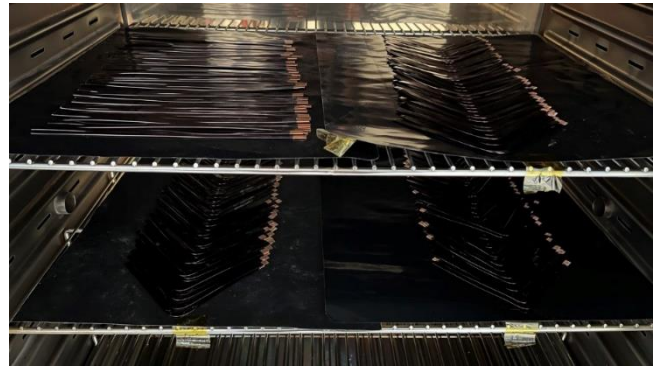
Fig. 5. Edgewise insulated wires inside the oven before the accelerated thermal ageing process.
