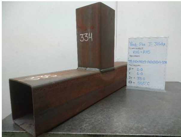
(b) Test vs FE comparison for RHS T-joint with \psi = 550^\circ\text{C} and failed by S mode.
