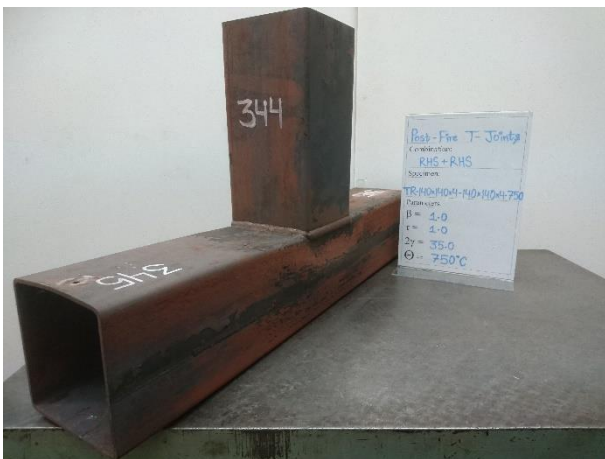
(c) Test vs FE comparison for RHS T-joint with \psi = 750^\circ\text{C} and failed by S mode.
