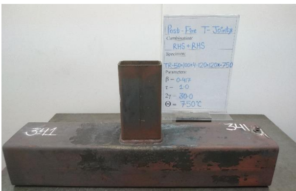
(c) Test vs FE comparison for RHS T-joint with \psi = 750^\circ\text{C} and failed by F mode.
