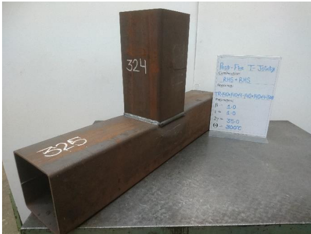
(a) Test vs FE comparison for RHS T-joint with \psi = 300^\circ\text{C} and failed by S mode.
