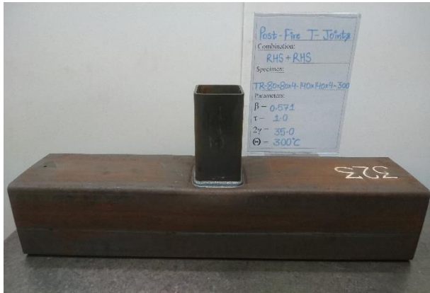
(a) Test vs FE comparison for RHS T-joint with \psi = 300^\circ\text{C} and failed by F mode.
