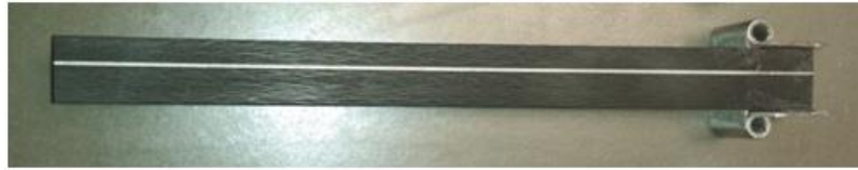
Figure 5. Ti-CFRP DCB sample designed taking into account the joint asymmetry
