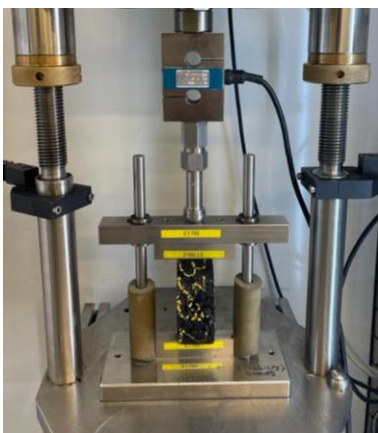
Figure 5. ITFT test configuration
