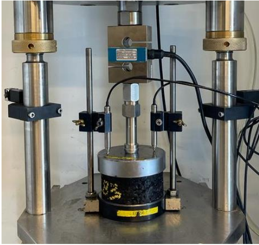
Figure 6. RLAT test configuration
