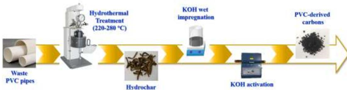
**Figure 1 Schematic diagram of PVC hydrochar derived activated carbons**
