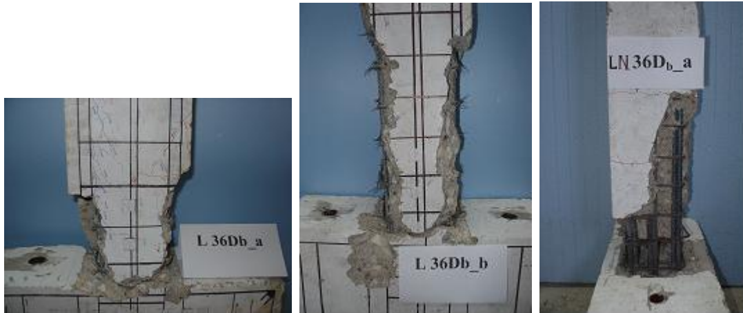
Figure 6 Specimens with lap-splices after removing the loose concrete fragments
