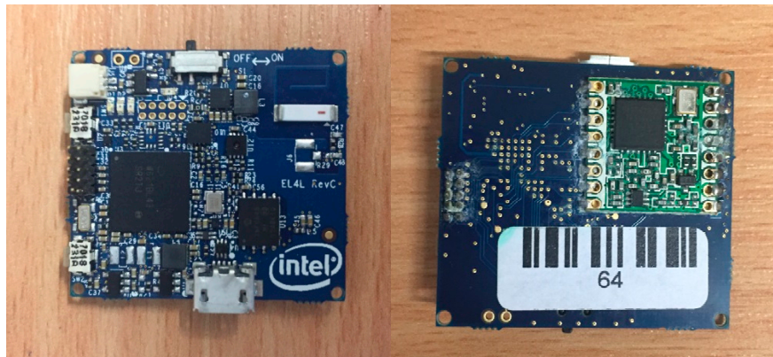
Figure 7. Custom-made device (including processor, memory, radio, inertial measurement unit (IMU), etc.).
