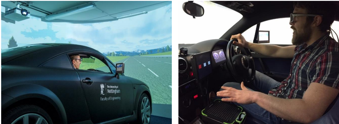
Figure 1. Medium-fidelity driving simulator showing motorway scenario (left) and participant interacting with mid-air haptics (right), with transducer array (beneath hand), Leap Motion camera (beneath wrist) and visual (touchscreen) display with button 'one' of three selected (in red).
