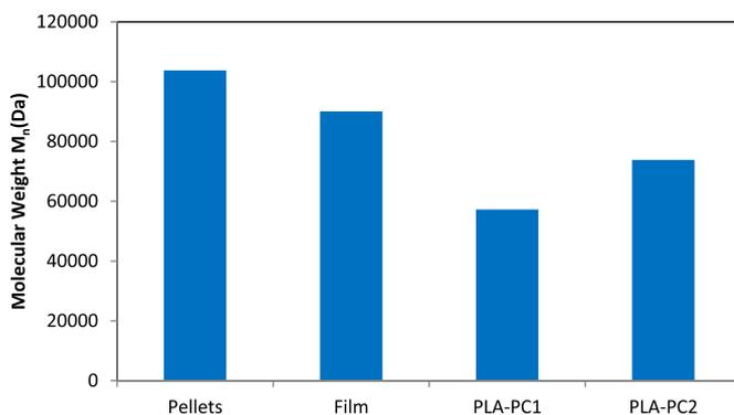
Fig. 7. Molecular weight of PLA pellets, films, and PLA plates produced under two different processing conditions (PLA-PC1 and PLA-PC2). Errors were within 0.3% (Gel permeation chromatogr, 2007).
