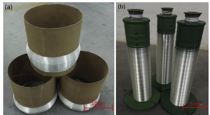
Fig. 1. (a) cakes with fibre strands; (b) yarns wound on milk-bottle bobbins.
