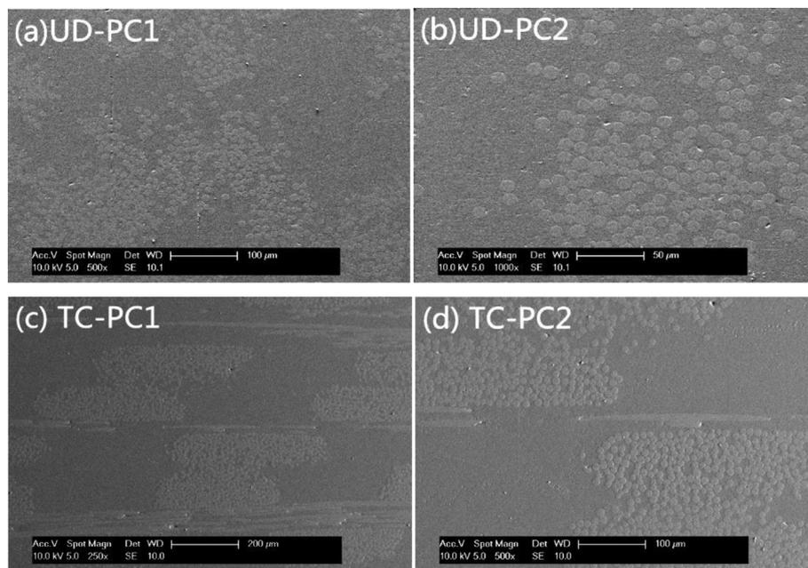
Fig. 6. The SEM micrographs of the cross sections of composites: (a) UD-PC1; (b) UD-PC2; (c) TC-PC1; (4) TC-PC2.
