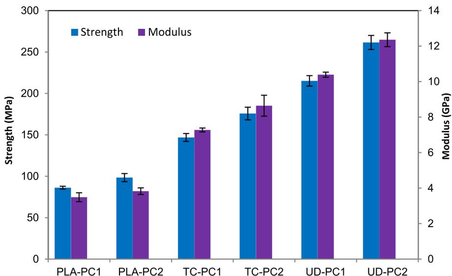
Fig. 3. Flexural strength and modulus of PLA, textile and UD composite plates, produced using two different processing conditions during compression moulding.
