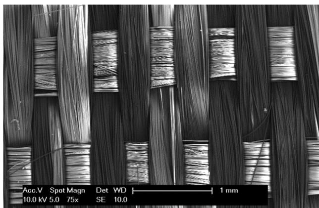
Fig. 5. SEM image of the PGF textile surface. No gaps were seen between adjacent yarns and few broken fibres were observed.
