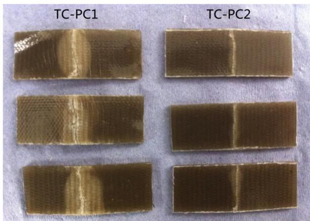
Fig. 4. Textile composites (TC-PC1 and TC-PC2) after flexural tests. Delamination was seen for TC-PC1.
