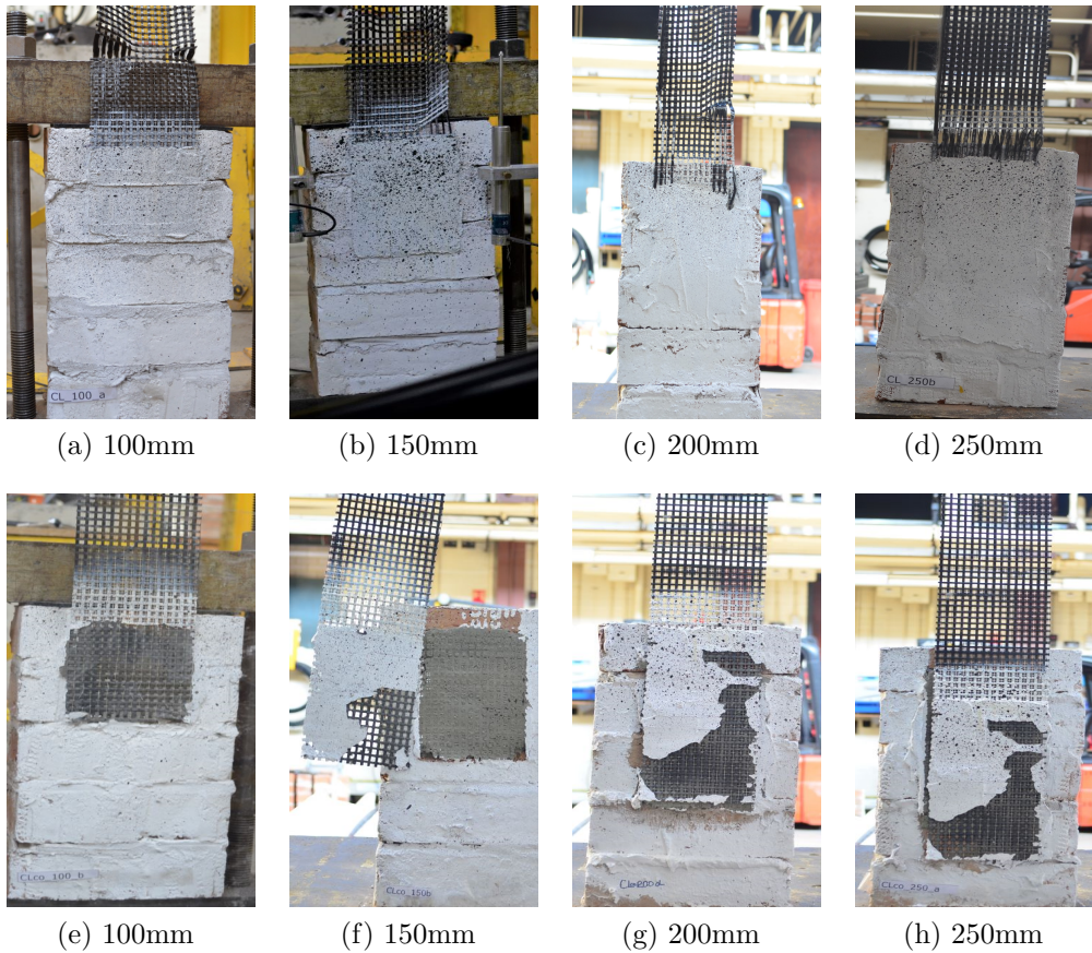
Figure 10: Typical failure modes of specimens strengthened with light carbon textile: (a)-(d) uncoated specimens, failure mode: Textile slippage; (e)-(h) coated specimens, failure mode: detachment.
