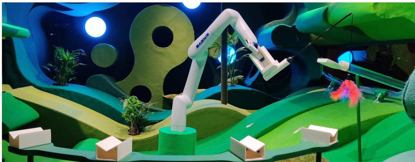
Figure 1: View of the environment with the Kinova robot at the centre and the end-effector attachment rack in the front.
